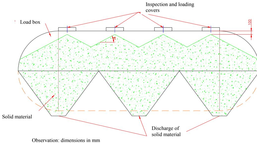
Figure 12. Graphical determination of the amount of inspection covers.
