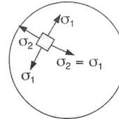
Figure 9. Principal stresses for a cylindrical vessel      Figure 10. Principal stresses for a spherical vessel
