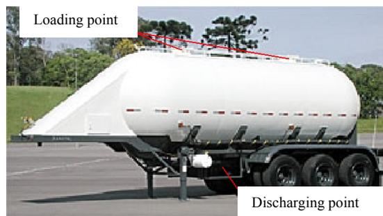
Figure 1. Road silo semitrailer (Randon, 2004).
