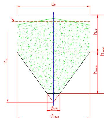
Figure 14. Main dimensions of a module.
