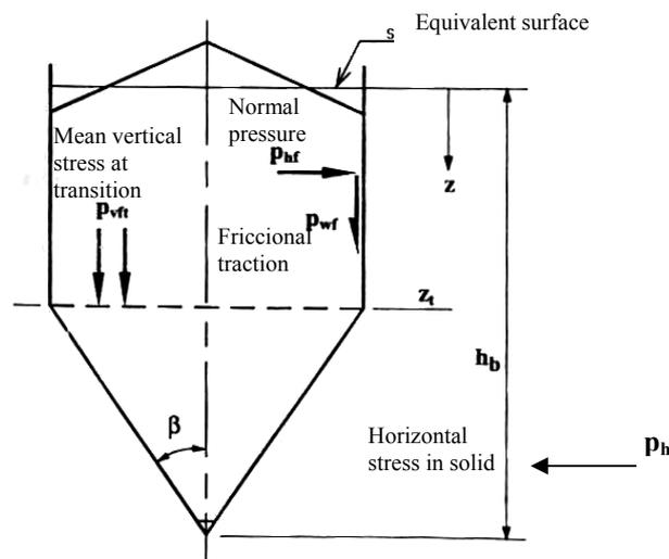
Figure 3. Pressures in barrel after filling (Rotter, 2001)
