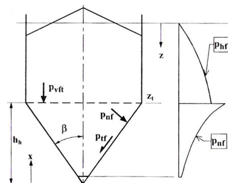
Figure 8. Filling pressures on steep conical hopper walls (Rotter, 2001).
