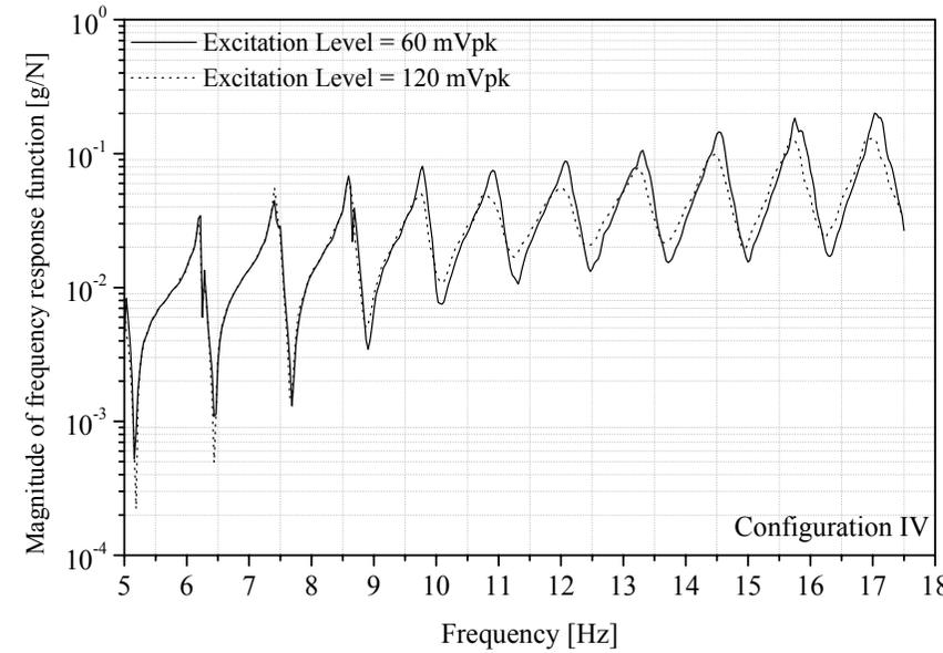
Figure 4. Magnitude of the frequency response function at the driving point for the four configurations tested and for two excitation levels: 60 mVpeak and 120 mVpeak.
