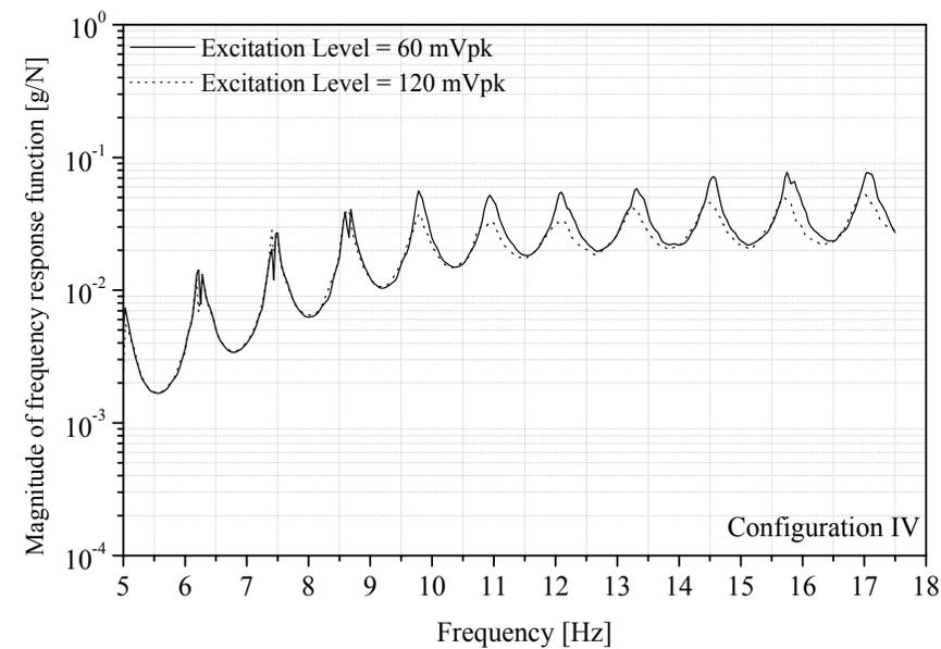
Figure 6. Magnitude of the frequency response function at  $x = 0.70$  m for the four configurations tested and for two excitation levels: 60 mVpeak and 120 mVpeak.
