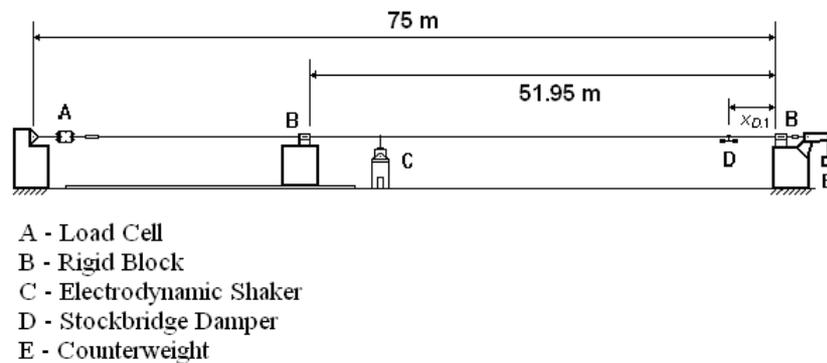
Figure 2. Schematic view of the experimental apparatus for the laboratory tests performed.
