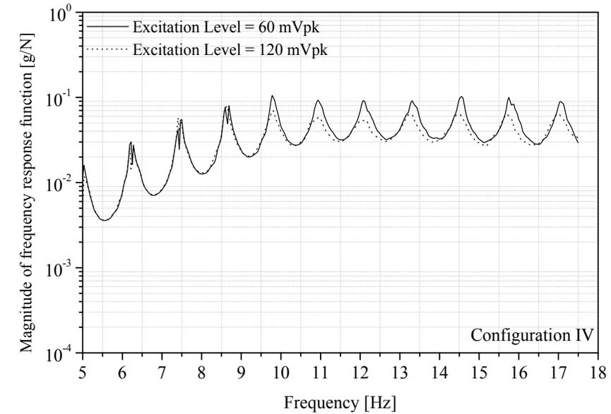
Figure 5. Magnitude of the frequency response function at  $x = 1.39$  m for the four configurations tested and for two excitation levels: 60 mVpeak and 120 mVpeak.
