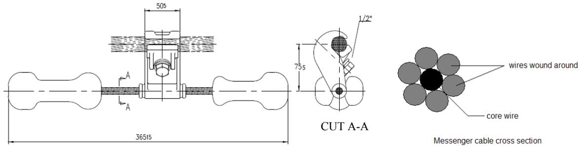
Figure 3. The Stockbridge damper used in the laboratory tests.
