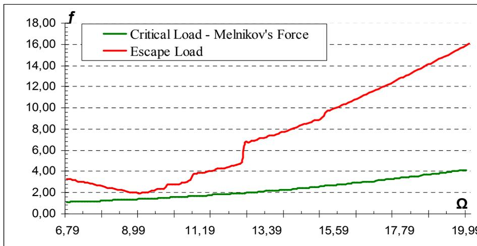
Figure 5. Comparison between the loads for  $0.5 \omega_0 < \Omega \text{ (rad/s)} < 1.5 \omega_0$  considering the Eq. (24).
