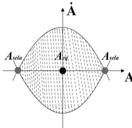
Figure 2. Basin of attraction of the column's model defined by Fig. (1) and Eq. (1).
