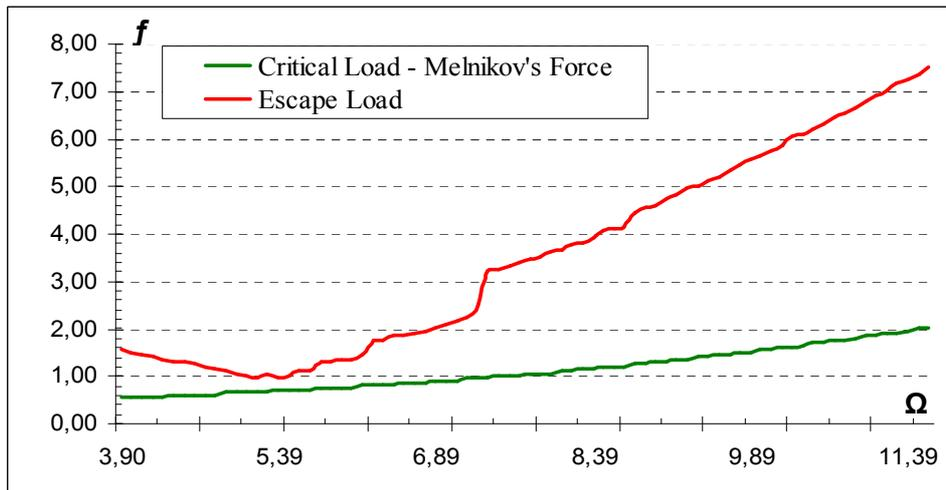
Figure 4. Comparison between the loads for  $0.5 \omega_0 < \Omega \text{ (rad/s)} < 1.5 \omega_0$  considering the Eq. (23).
