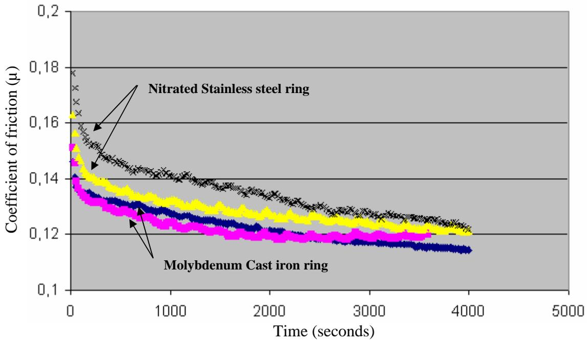
Figure 8. Stabilization of friction coefficient before long tests.
