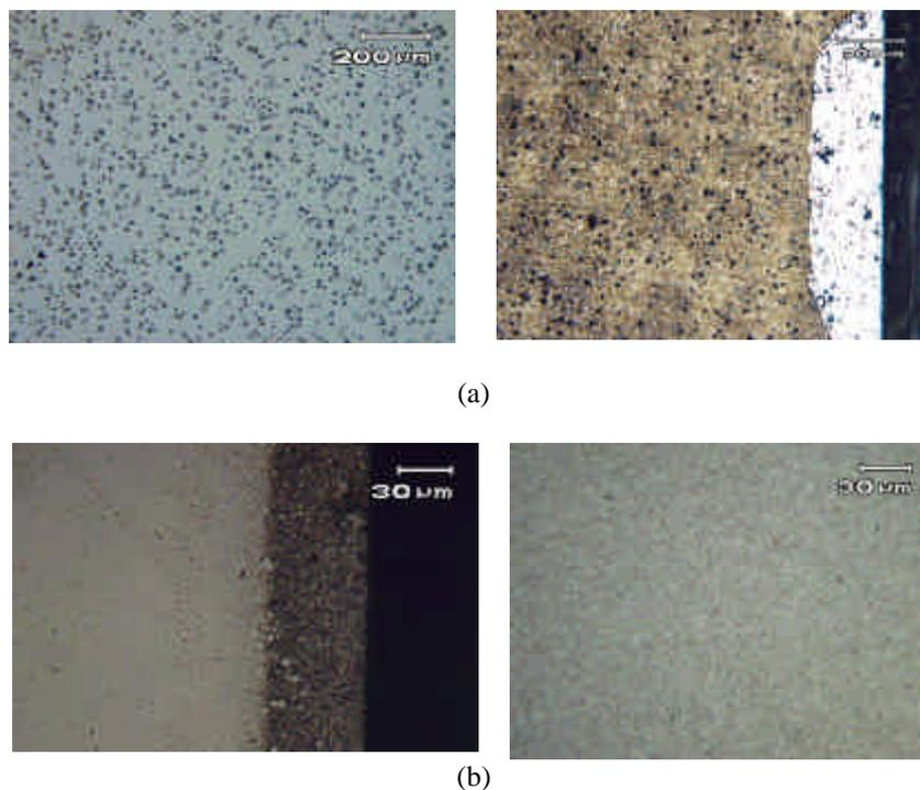
Figure 2. Microstructure photographs on piston ring coating and structure. (a) Martensitic ductile iron and molybdenum thermal plasma coating 100 X (Without and with nital attack). (b) Nitrided layer of depth with 70 mm in martensitic stainless steel. 500 X (Vilela attack).
