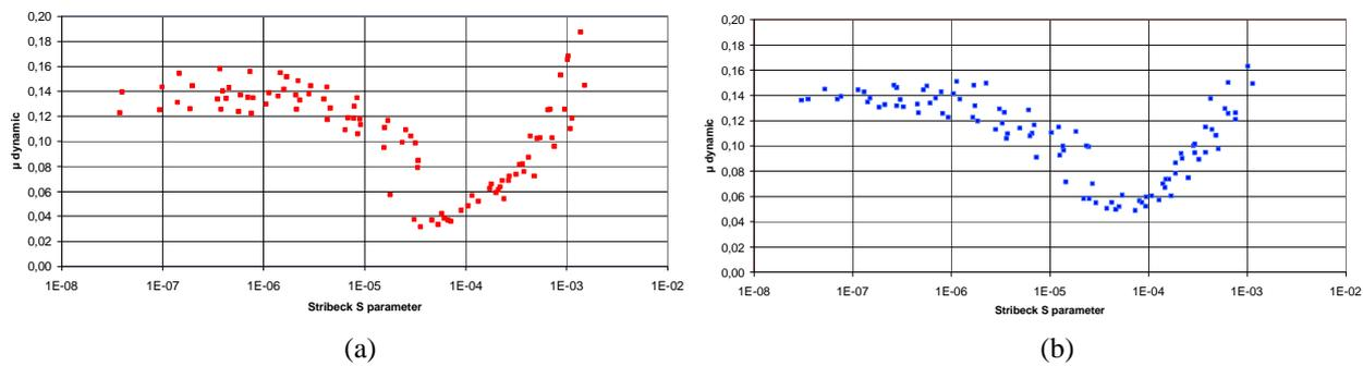
Figure 4. Variation of friction coefficient and Stribeck parameter of Cast iron ring (a) and Stainless steel ring (b) against cast iron cylinder liner segment with engine oil grade 10W40.
