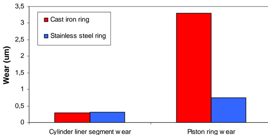
Figure 9. Wear in cylinder segment liner and piston ring surfaces after 48h of sliding conditions.
