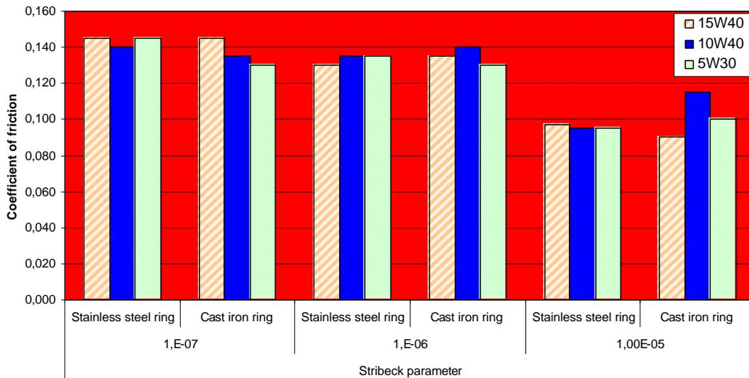
Figure 7. Average values for boundary and mixed phase of Stribeck curve.
