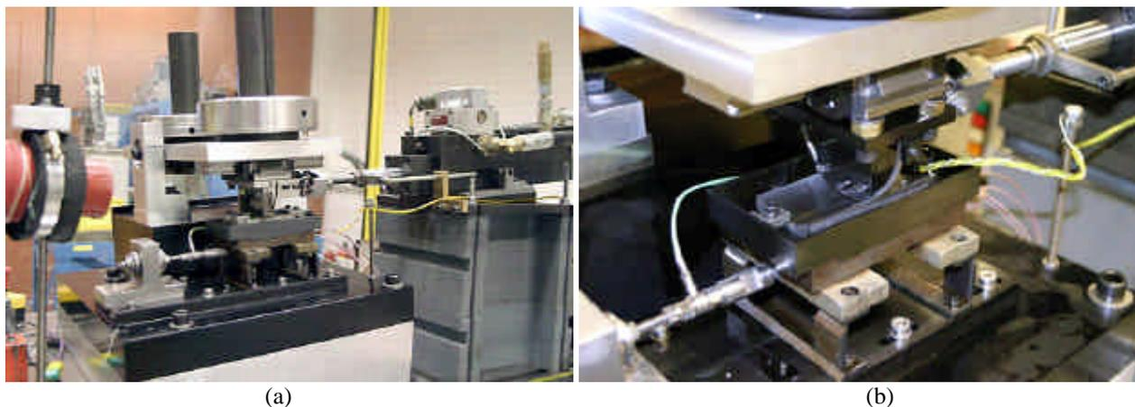
Figure 1. Picture of reciprocating friction machine (a) and piston ring assembly.
