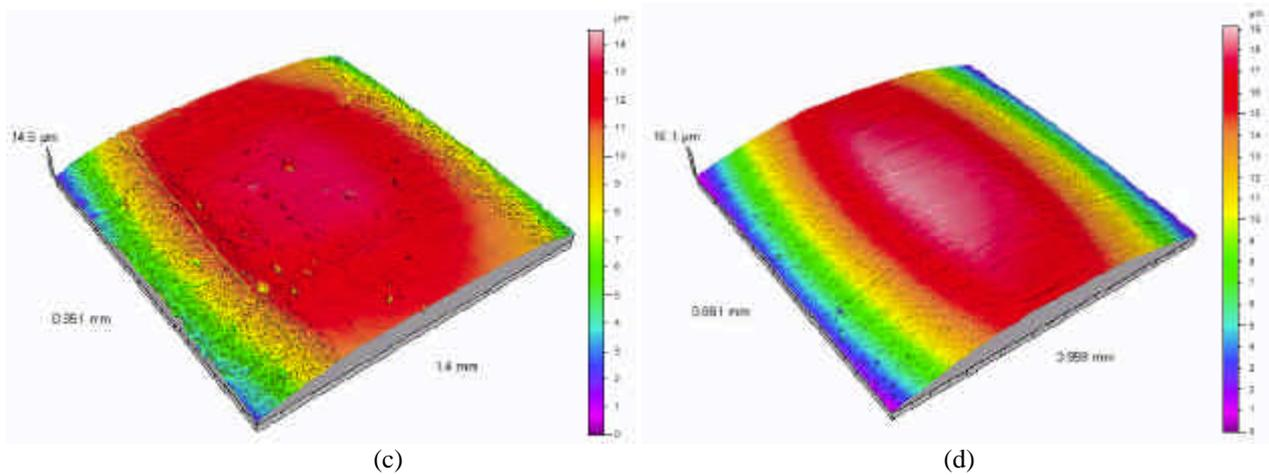
Figure 11. Cartographies 3D of cast iron piston ring (c) and stainless steel piston ring (d) with the values of surface wear.
