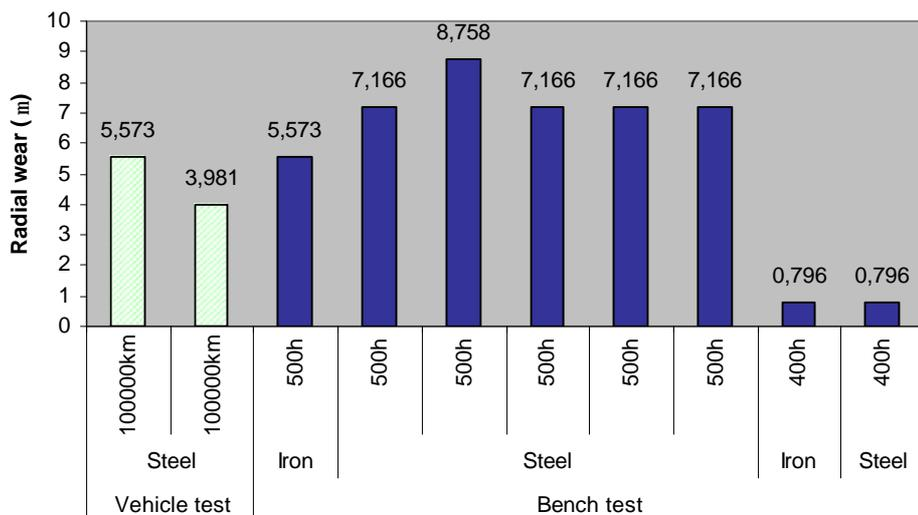
Figures 12. Values of radial wear in stainless steel and cast iron rings running in vehicle and bench tests.
