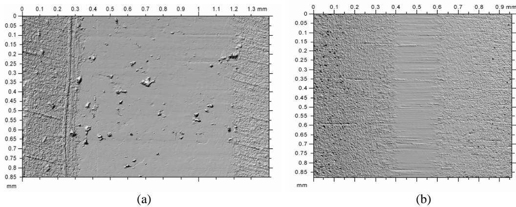
Figure 10. Width of contact in cast iron piston ring (a) and stainless steel piston ring (b) after 48h of test.
