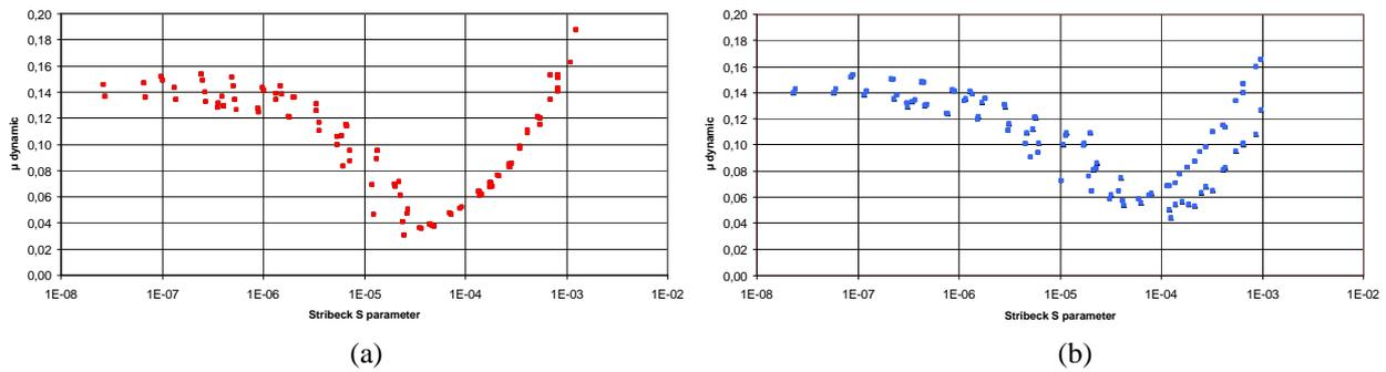
Figure 3. Variation of friction coefficient and Stribeck parameter of Cast iron ring (a) and Stainless steel ring (b) against cast iron cylinder liner segment with engine oil grade 15W40.
