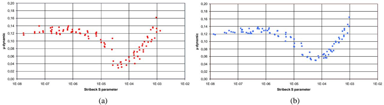
Figure 5. Variation of friction coefficient and Stribeck parameter of Cast iron ring (a) and Stainless steel ring (b) against cast iron cylinder liner segment with engine oil grade 5W30.
