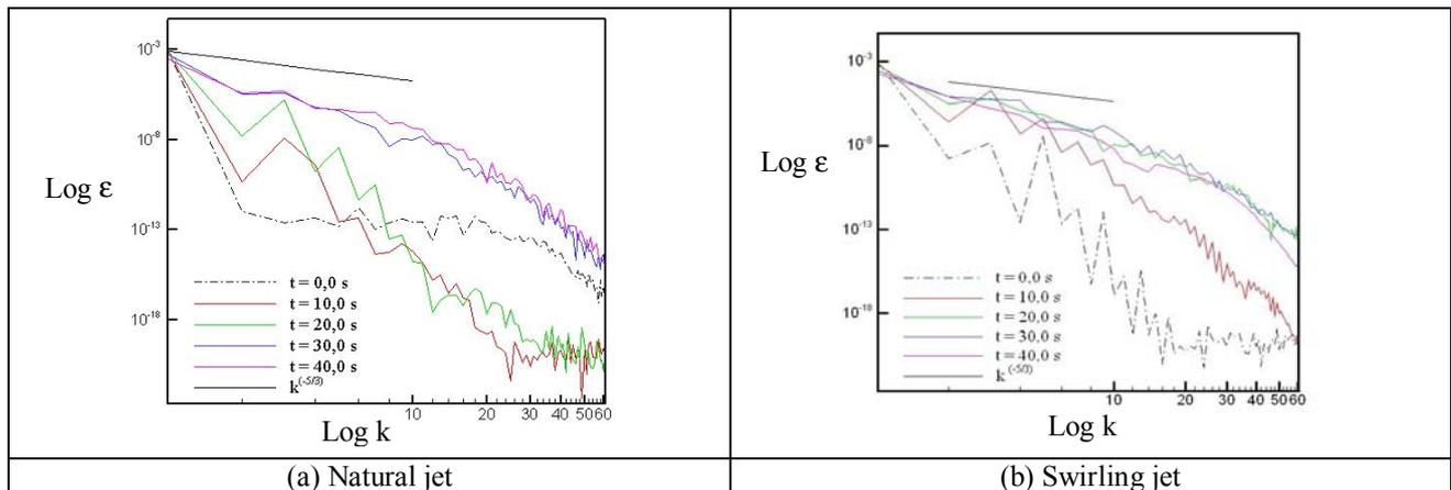
Figure 11. Turbulent Kinetic Energy Spectrum for Natural and Swirling Jets.
