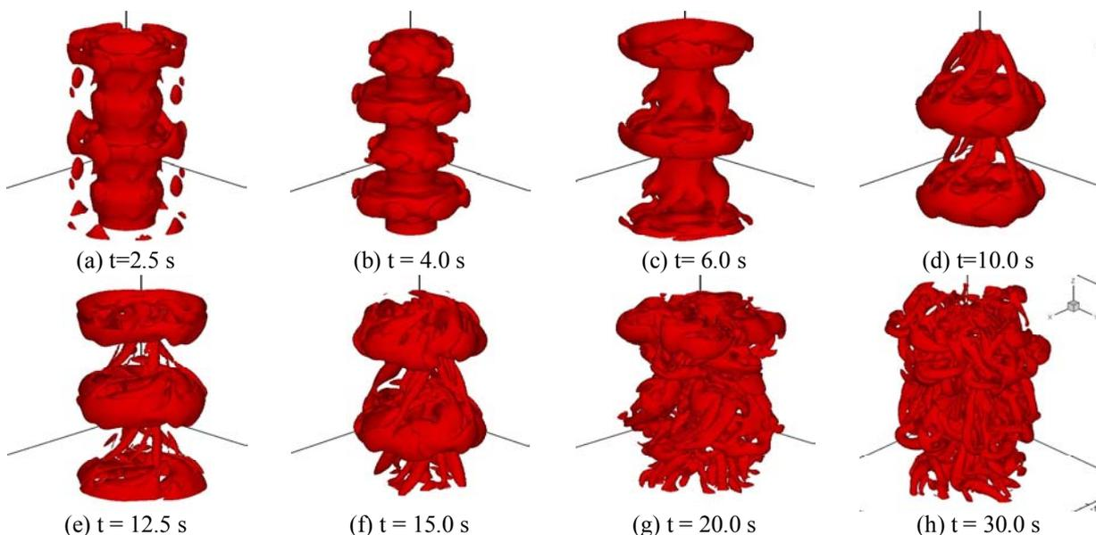
Figure 2. Criterion  $Q$  temporal evolution (Isosurface level =  $0.01 \text{ s}^{-2}$ ) - Swirling Jet.
