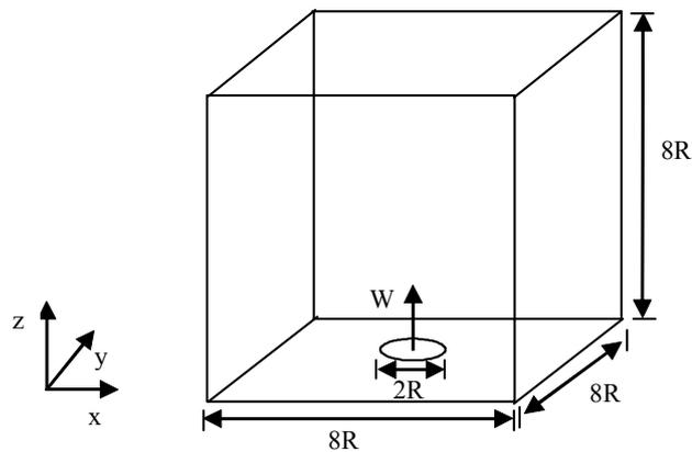
Figure 1. Scheme of computational domain.
