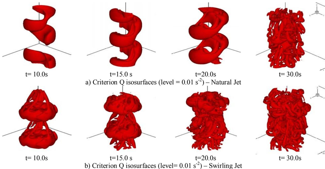
Figure 10. Comparison of temporal evolution through criterion Q isosurfaces between Natural and Swirling jets.
