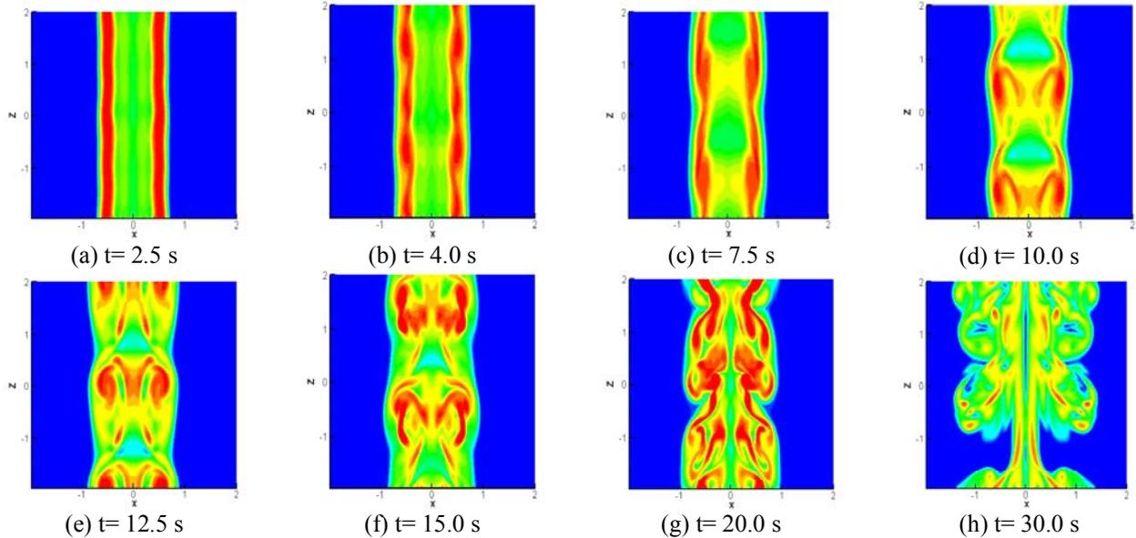
Figure 3. Vorticity  $\|\bar{\omega}\|$  in temporal evolution in the plane  $xz$  ( $y=0$ ) – Swirling Jet.
