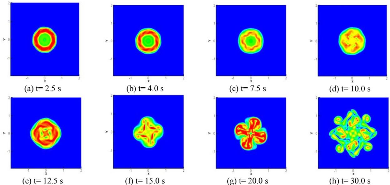
Figure 4. Vorticity  $\|\bar{\omega}\|$  in temporal evolution in the plane  $xy$  ( $z=0$ ) – Swirling Jet.
