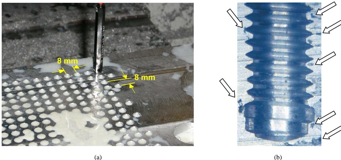
Figure 5. General view of the work material after machined some threaded holes (a) and transverse section of the machined work-piece after 5,691 threads holes (b). The details of the material porous are indicated by arrows.
