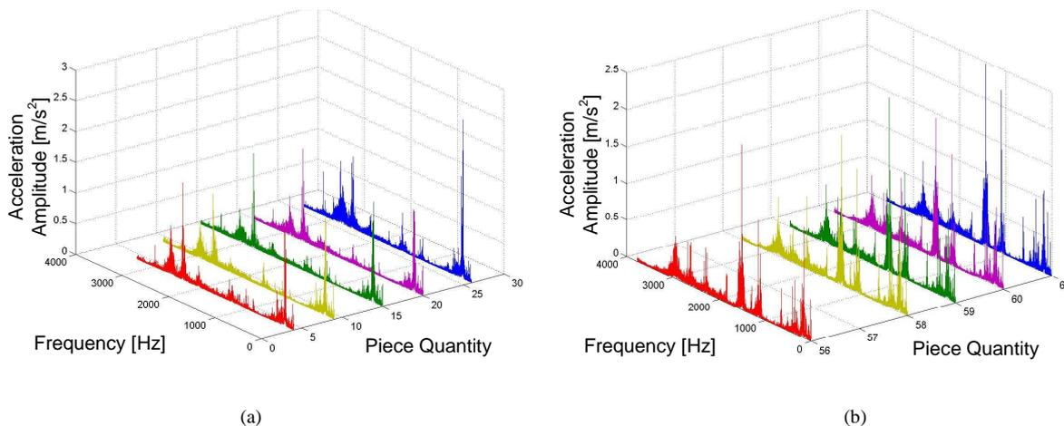
Figure 10. Acceleration of vibration on frequency spectra – fixture system using four bolts in (a) from 1,980 to 12,870 threaded holes and in (b) from 27,720 to 30,253 threaded holes.
