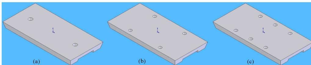
Figure 4. Models of fixture systems for FEM evaluation using: a) 2; b) 4; and c) 6 bolts.
