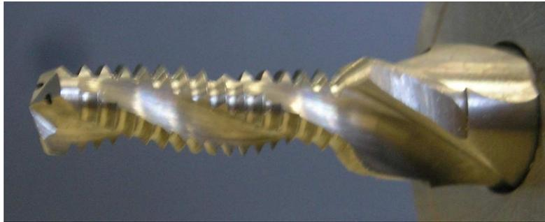
Figure 1. Tap mill tool (diameter of 5 mm and length of 65 mm).
