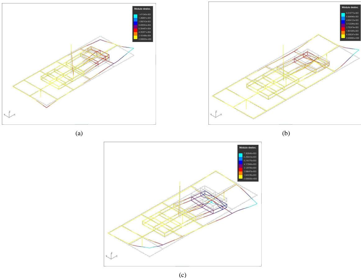
Figure 7. Maximum displacements for excitation of spindle: rotation of 7,333 rpm (a), 8,000 rpm (b), and 9,333 rpm (c).
