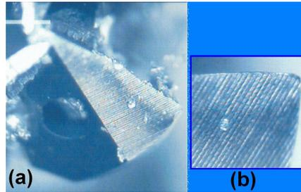
Figure 6. View of the tool after 5,691 thread holes were machined (a) and detail of the tool rake face (b).
