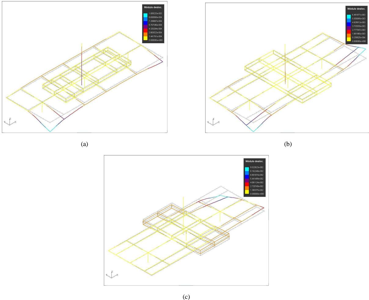
Figure 8. Maximum displacements for fixture system using 2 bolts (a), 4 bolts (b), and 6 bolts (c) – ODS analysis.
