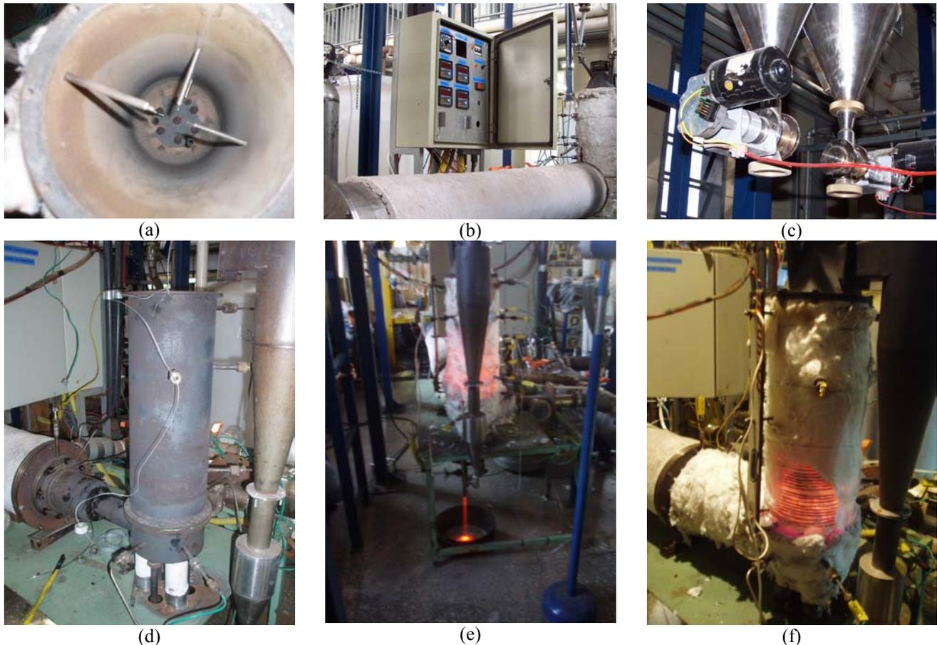
Figure 2. (a) Internal view of reactor; (b) air heater, reactor and control panel; (c) feeding valves of coal and limestone; (d) reactor out of operation; (e) and (f) reactor in operation.
