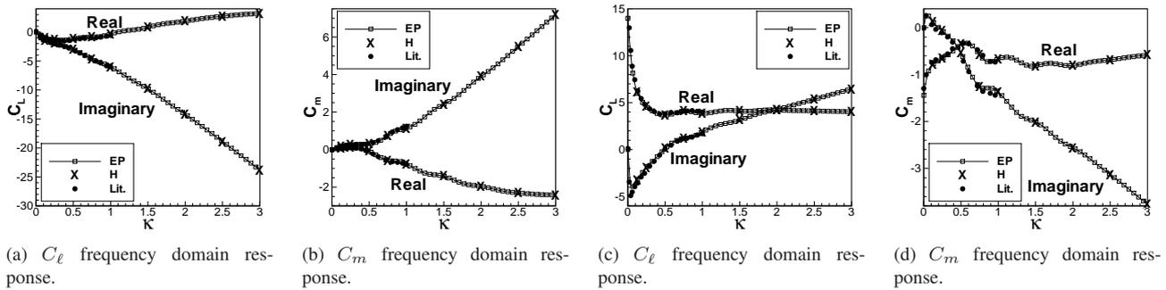
Figure 1. Low reduced frequency response of a NACA 0012 airfoil at  $M_\infty = 0.80$  and  $\alpha_0 = 0$  to an impulsive input.
