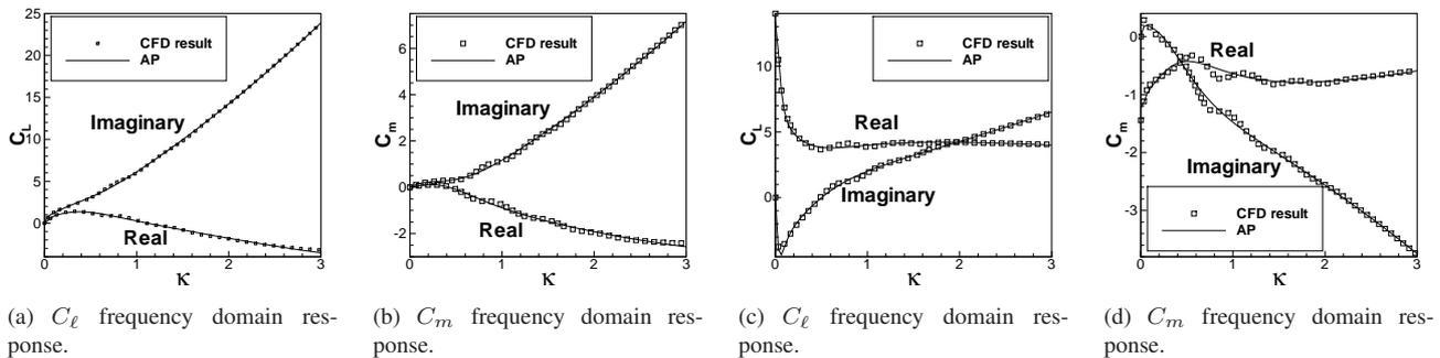
Figure 2. Low reduced frequency response of a NACA 0012 airfoil at  $M_\infty = 0.80$  and  $\alpha_0 = 0$  to an impulsive input. Comparisons between CFD results and approximated data.
