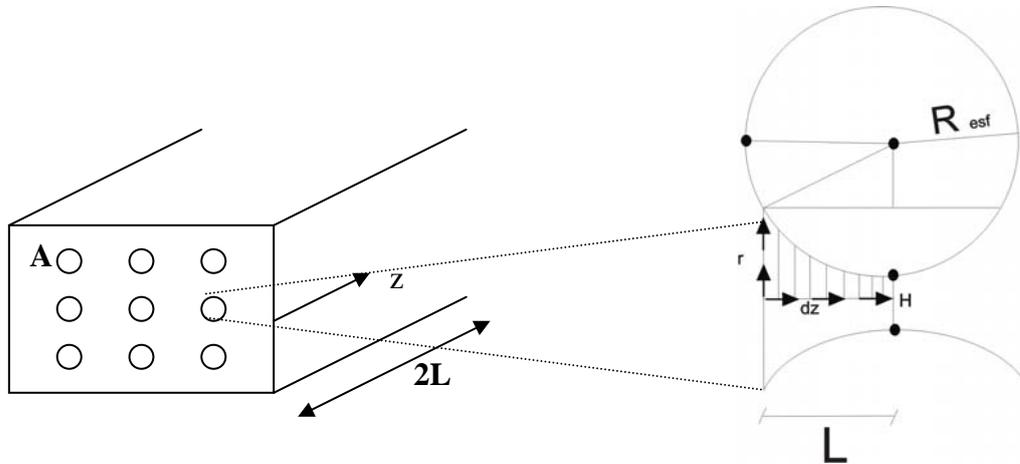
Figure 1.1 – Schematic of the idealized porous media.
