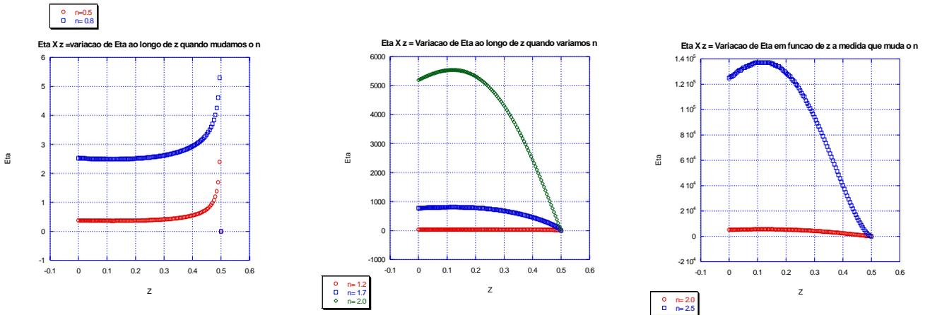
Figure 4.2 – Variation of viscosity with the longitudinal position  $z$  (a) comparison between two viscosity-thinning fluids,  $n=0.8$  and  $n=0.5$ , (b) comparison between three viscosity-thickening fluids,  $n=1.2$ ,  $n=1.7$ , and  $n=2.0$ ; (c) comparison between two viscosity-thickening fluids,  $n=2.0$  and  $n=2.5$ .
