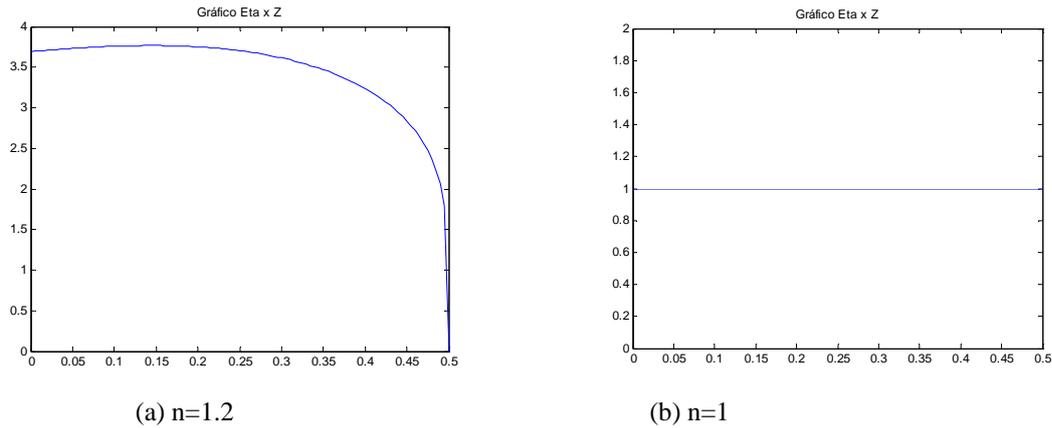
Figure 4.1 – Variation of viscosity with the longitudinal position  $z$  (a) for an extensional power-law model with the behavior index  $n = 1.2$ ; (b) for a Newtonian fluid.
