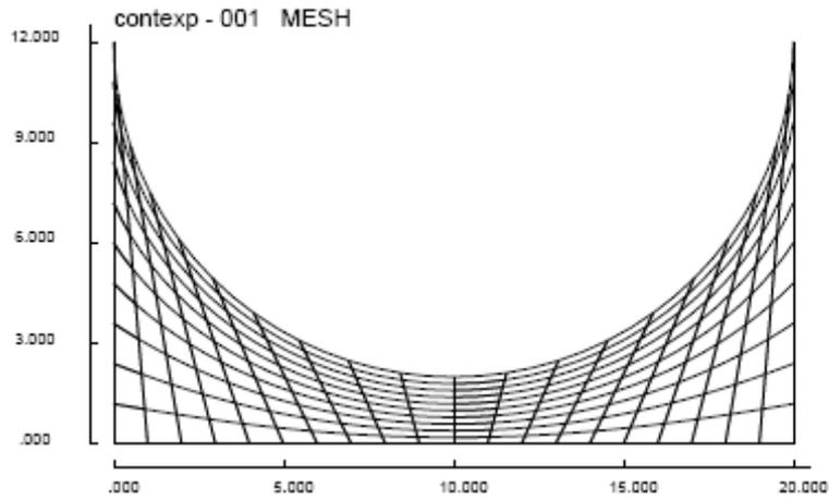
Figure 3.1 – Representative mesh of the half of the domain indicated in Figure 1.1
