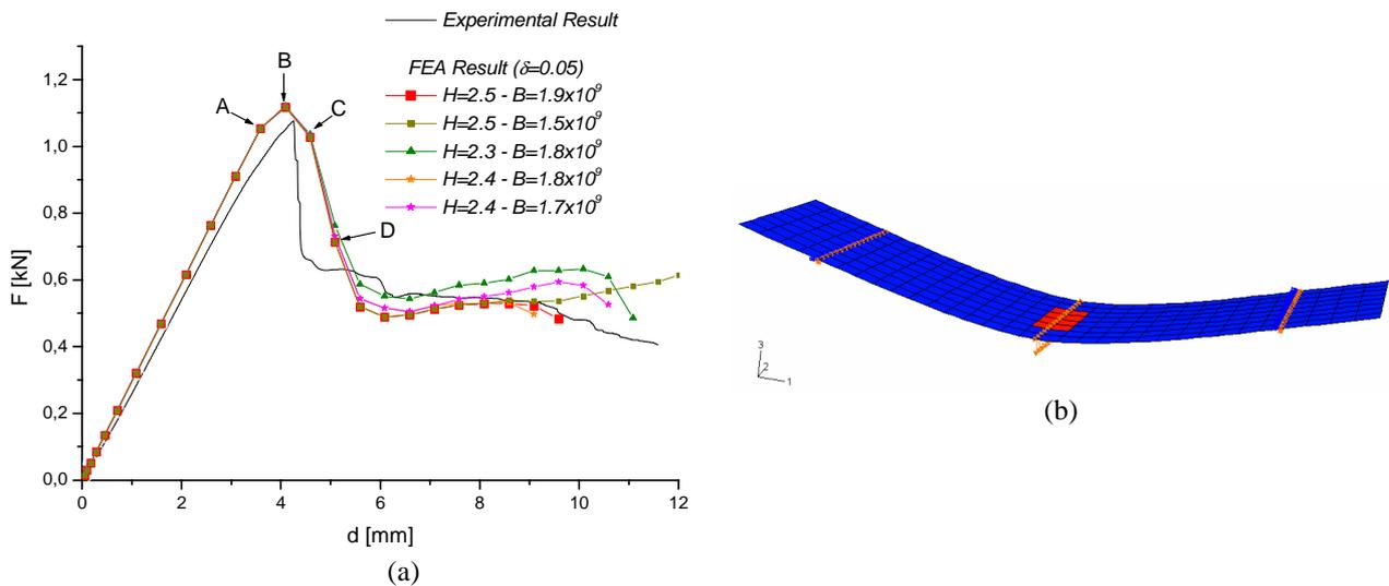
Figure 6. (a) Numerical and experimental results for laminate  $[0]_{10}$ ; (b) First failure elements
