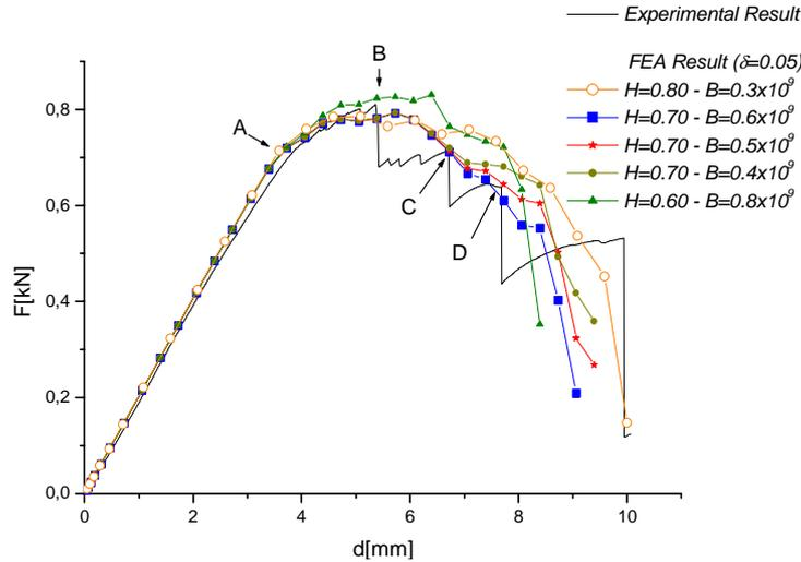
Figure 8. Numerical and experimental results for laminate  $[0/90/0/90/0]_s$
