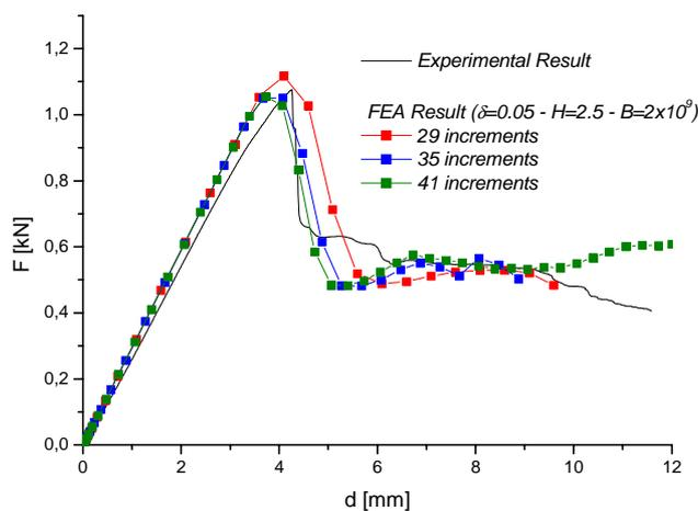
Figure 7. Test of increment numbers for laminate  $[0]_{10}$
