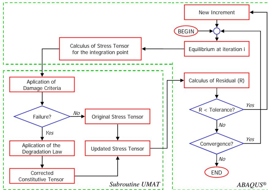
Figure 5. UMAT subroutine and software ABAQUS™.
