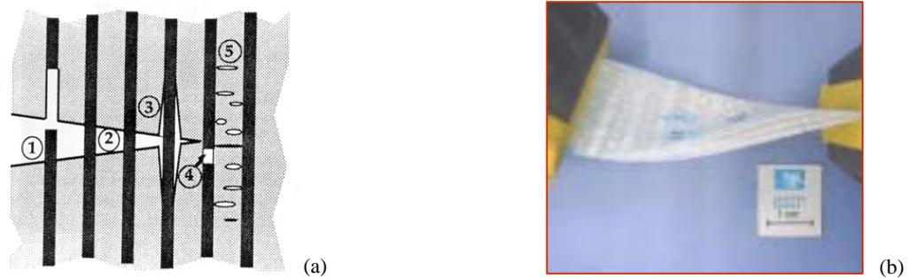
Figure 1. Composite failure mechanisms: (a) intra-ply (Anderson, 1995); (b) inter-ply failures (delamination)
