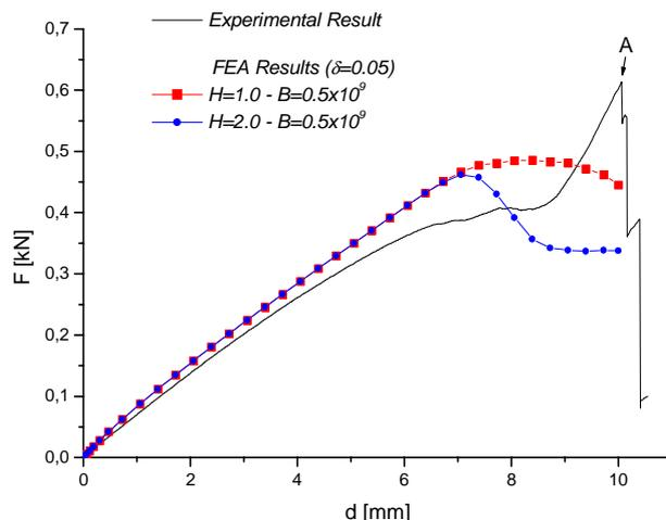
Figure 9. Numerical and experimental results for laminate [+45/-45/+45/0/90]<sub>s</sub>
