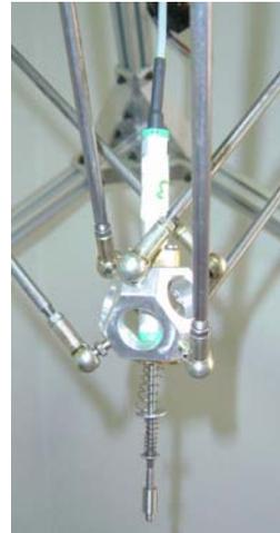
(b) End-effector with a linear transducer.
