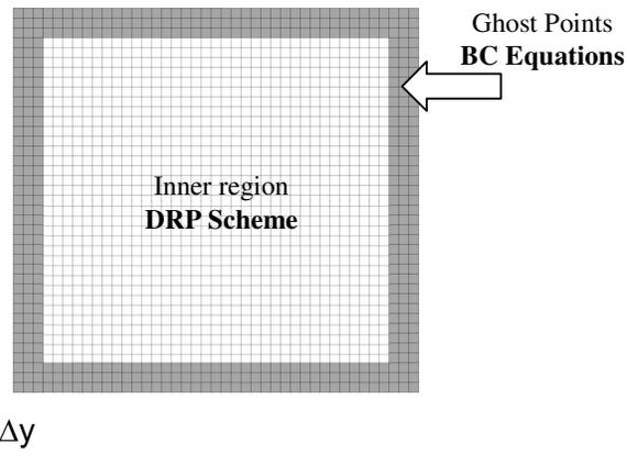
**Figure 2 - Computational domain and numerical parameters.**
