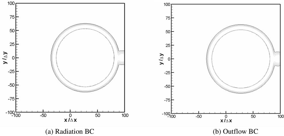
**Figure 6** – Density contours at 1100 time steps - Comparison between Radiation and Outflow BC's.
