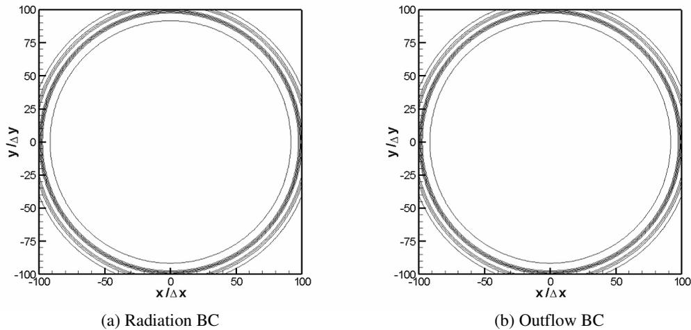
**Figure 4** – Pressure contours at 2000 time steps – Comparison between Radiation and Outflow BC's.
