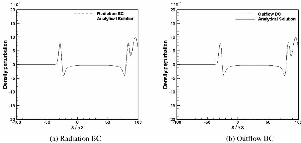
**Figure 7** – Density waveform along the centerline at 1100 time steps - Computed vs Analytical Solution for LEE.
