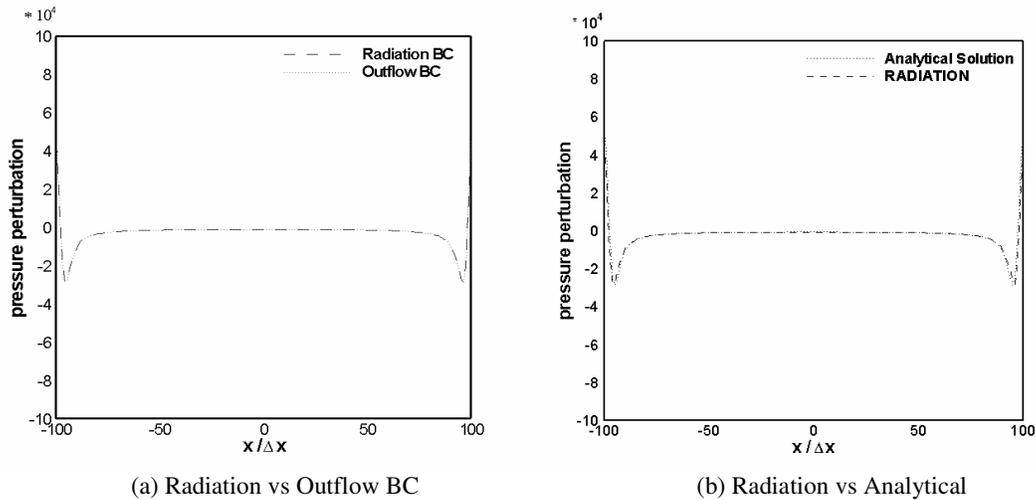
**Figure 5** – Pressure waveform along the centerline at 2000 time steps – Computed vs Analytical Solution for LEE.
