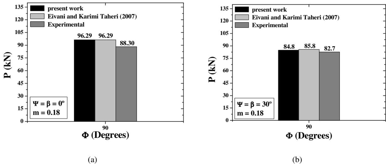
Figure 6. Predicted and measured ECAP loads obtained for an Al-6090: (a)  $\Psi = 0^\circ$  and (b)  $\Psi = 30^\circ$ .
