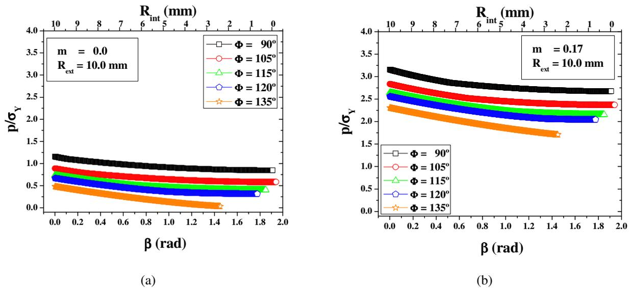
Figure 5. Normalized ECAP pressure as a function of geometrical parameters: (a)  $m = 0$  and (b)  $m = 0.17$ .
