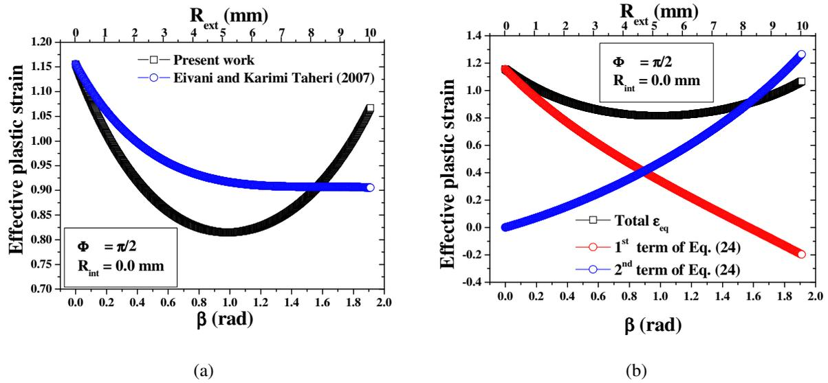
Figure 4. Effective plastic strain as a function of the outer die curvature angle  $\beta$  or the outer fillet radius  $R_{ext}$ : (a) comparison with the prediction determined with the model proposed by Eivani and Karimi Taheri (2007) and (b) terms of the present solution given by Eq. (24).
