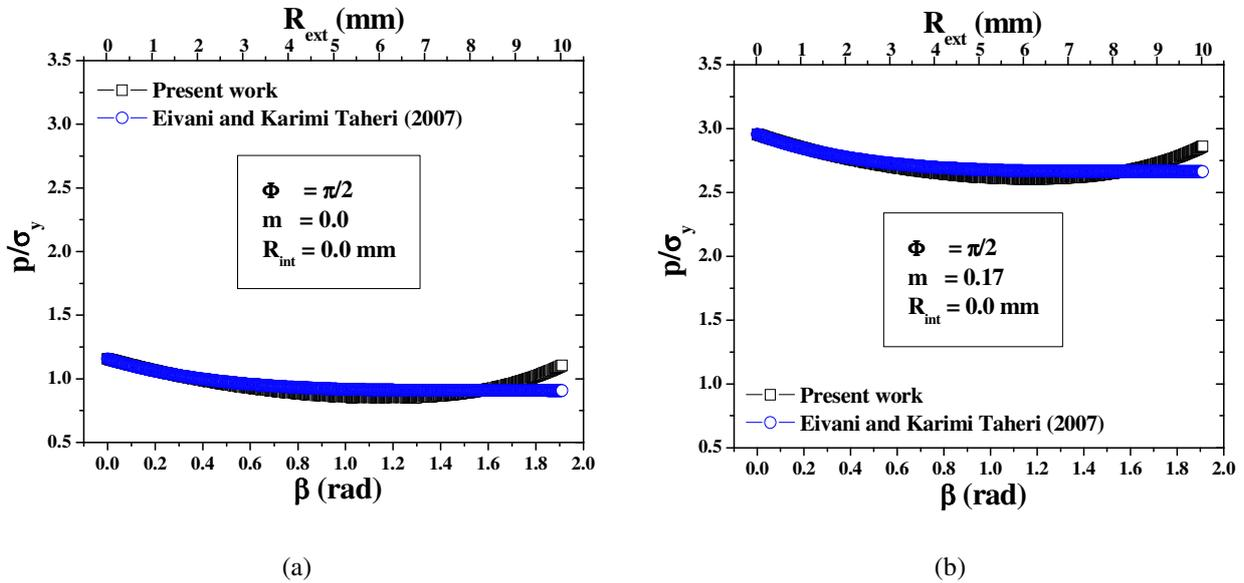
Figure 3. Normalized pressure determined for  $\Phi = \pi/2$  as a function of the angle  $\beta$ : (a)  $m = 0$  and (b)  $m = 0.17$ .
