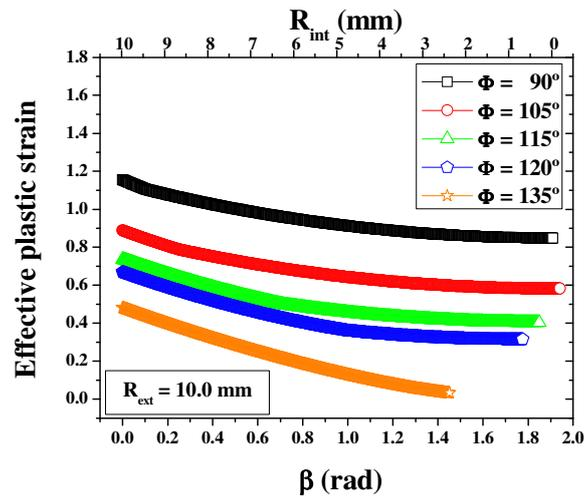
Figure 6. Effective plastic strains as a function of the  $\Phi$ ,  $R_{int}$  and  $\beta$ .
