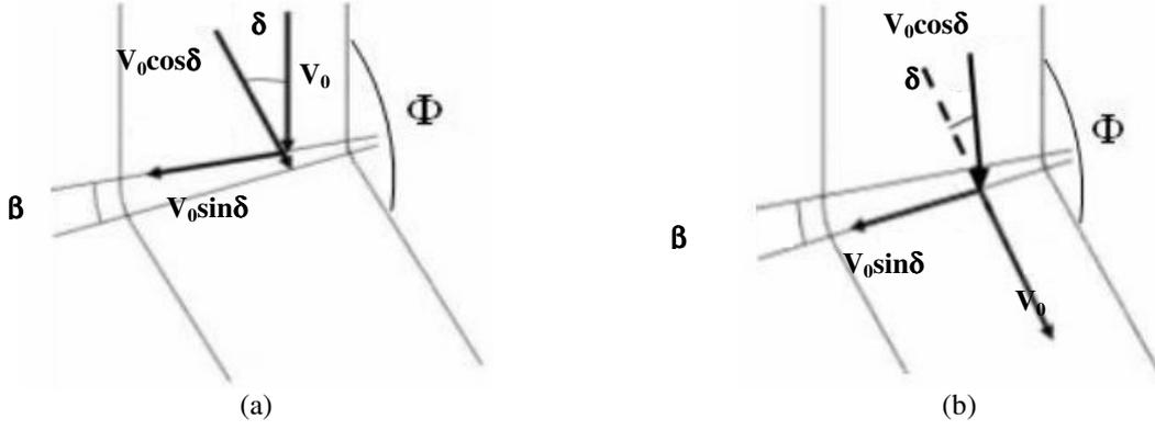
Figure 2. Velocity hodographs in the die deformation zone: (a) entry surface and (b) exit surface.
