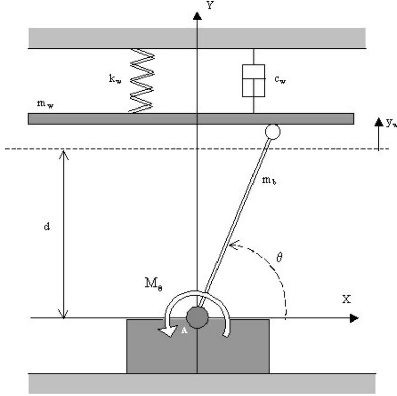
Figure 1. Rotating constrained bar.
