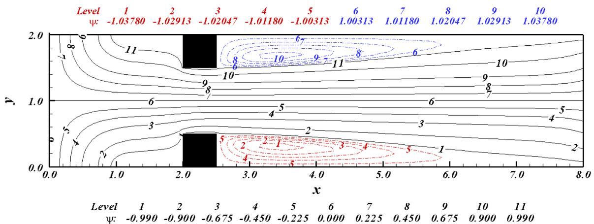
Figure 3. Stream function field ( $Re = 80$ ).
