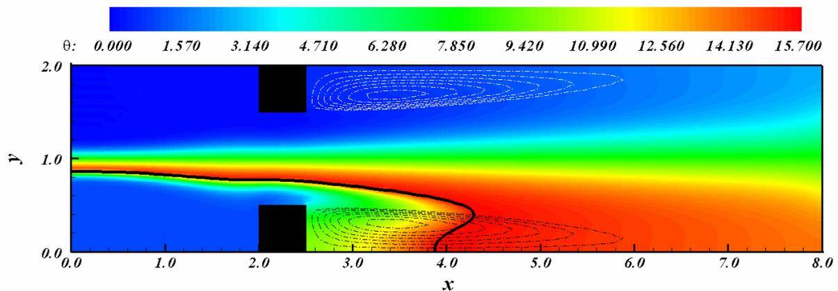
Figure 5. Temperature field ( $Re = 80$ ).
