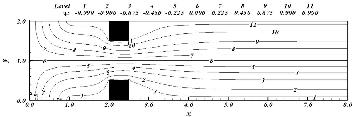
Figure 2. Stream function field ( $Re = 10$ ).
