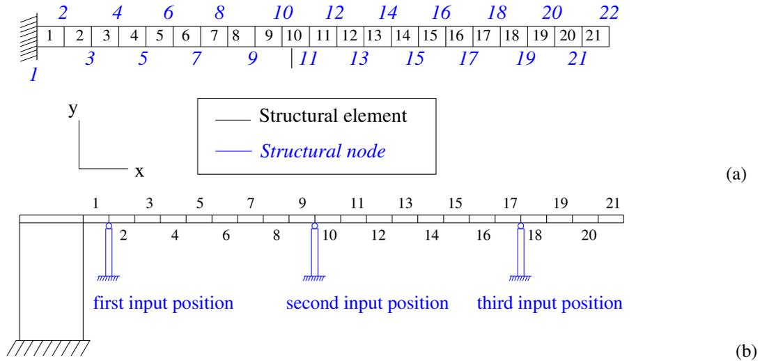
Figure 3. (a) structural nodes and elements; (b) input positions.
