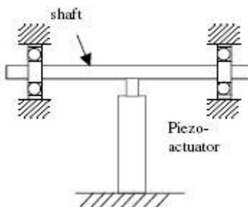
Figure 1. PZT stack acting on bearing supported shaft structure (Li et al., 2006).
