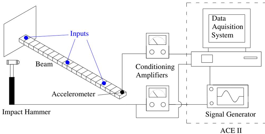
Figure 6. Disposition of experimental setup.
