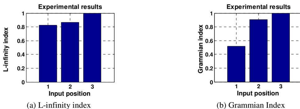
Figure 10.  $L_\infty$  and Grammian performance indices for the experimental tests.
