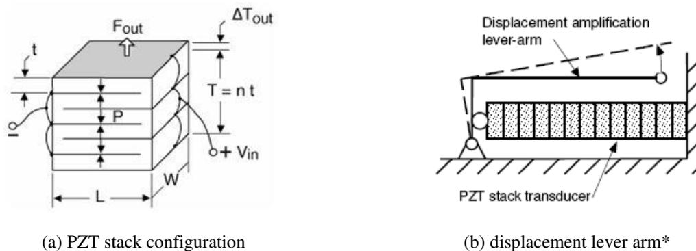
Figure 2. Illustration of a piezoelectric actuator stack.
