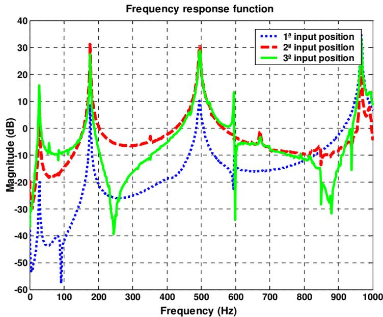
Figure 9. Frequency response functions for all three excitation positions.
