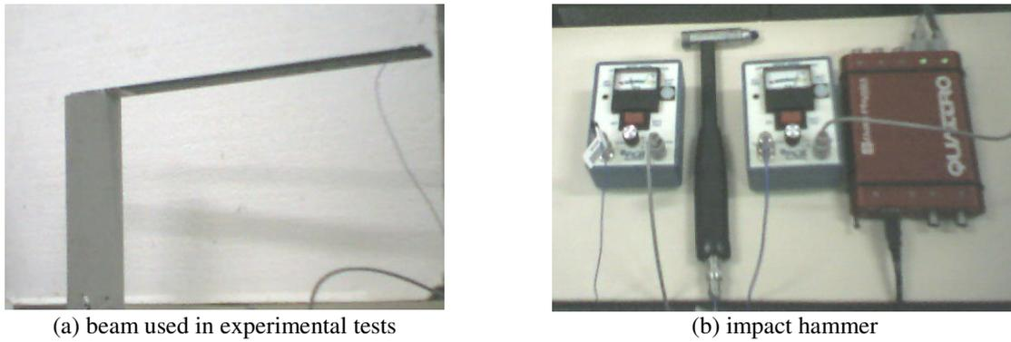
Figure 5. Cantilever beam and equipments used in experimental tests.
