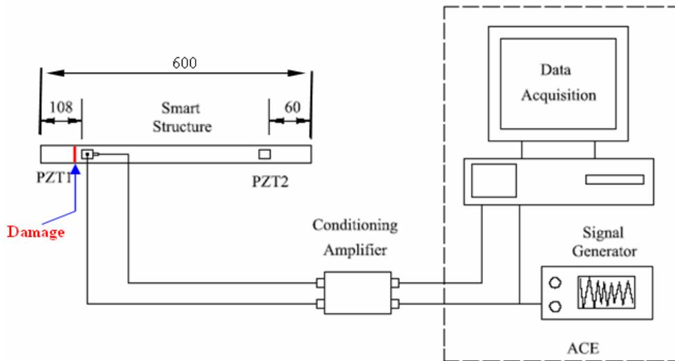
Figure 2. Schematic diagram of the measurement setup; dimensions in mm.
