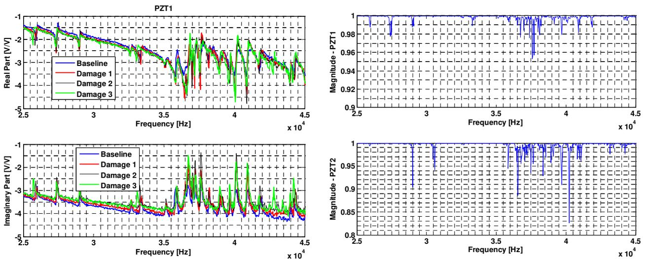
Figure 3. (a) Measurements in PZT1 for both healthy and damaged cases. (b) Magnitude squared coherence for PZT1 and PZT2 for the healthy condition.
