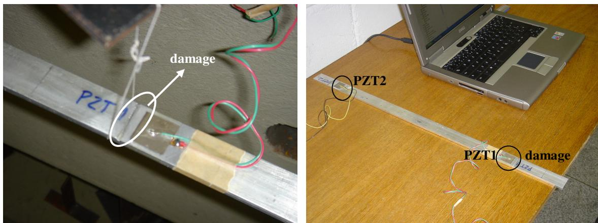
Figure 1. View of the smart beam used in the experimental tests. (a) PZT bonded in the smart beam and detail of the damage (transversal cut). (b) Smart beam with two bonded PZT patches.
