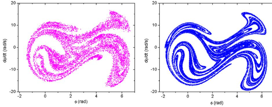
Figure 2. Chaotic strange attractors for  $\omega = 5.61$  rad/s . Experimental, left side, and numerical, right side.
