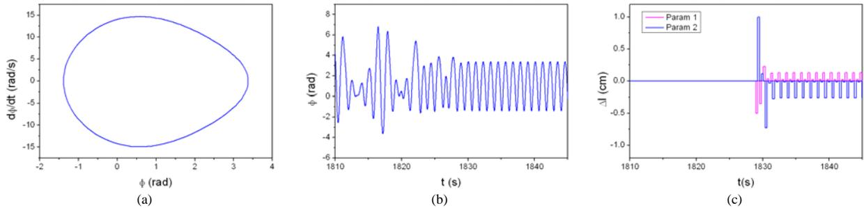
Figure 9. UPO period-1 stabilized using uncoupled approach: (a) Phase space; (b)  $\phi(t)$ ; (c)  $\Delta l_1(t)$  and  $\Delta l_2(t)$ .
