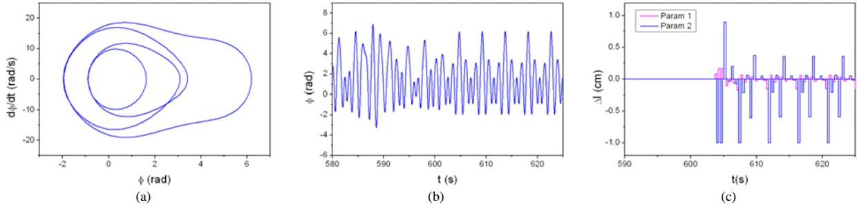
Figure 7. UPO period-4 stabilized using uncoupled approach: (a) Phase space; (b)  $\phi(t)$ ; (c)  $\Delta l_1(t)$  and  $\Delta l_2(t)$ .
