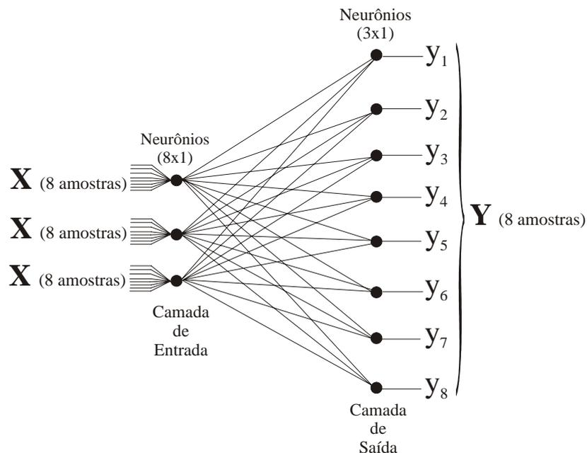
Figure 6. Representation of the MLNN used in the prediction.
