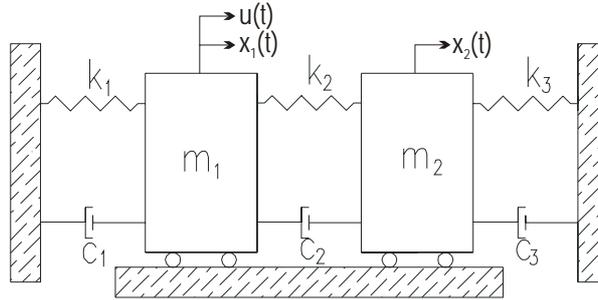
Figure 1. Representation of a 2DOF model
