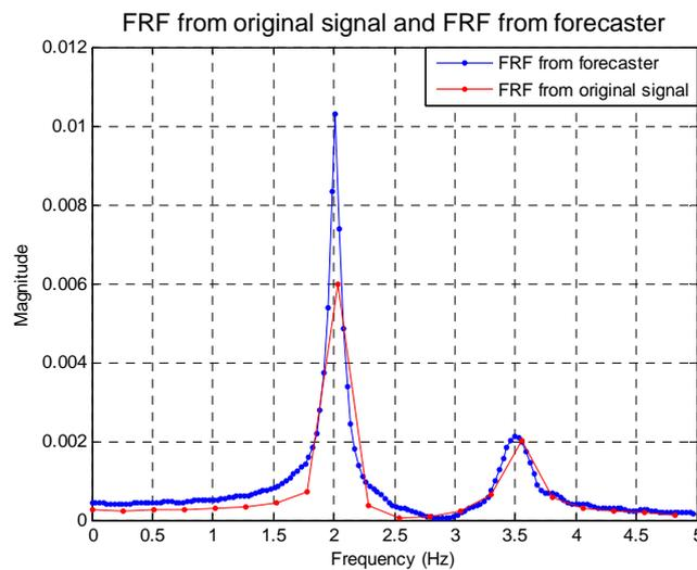
Figure 8. FRF estimate obtained from ARMAX predictor
