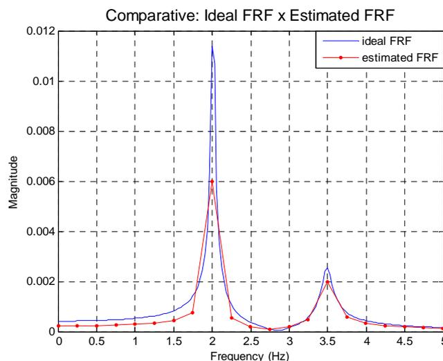
Figure 3. Comparison between the ideal FRF and estimate FRF from the signal obtained by simulation.
