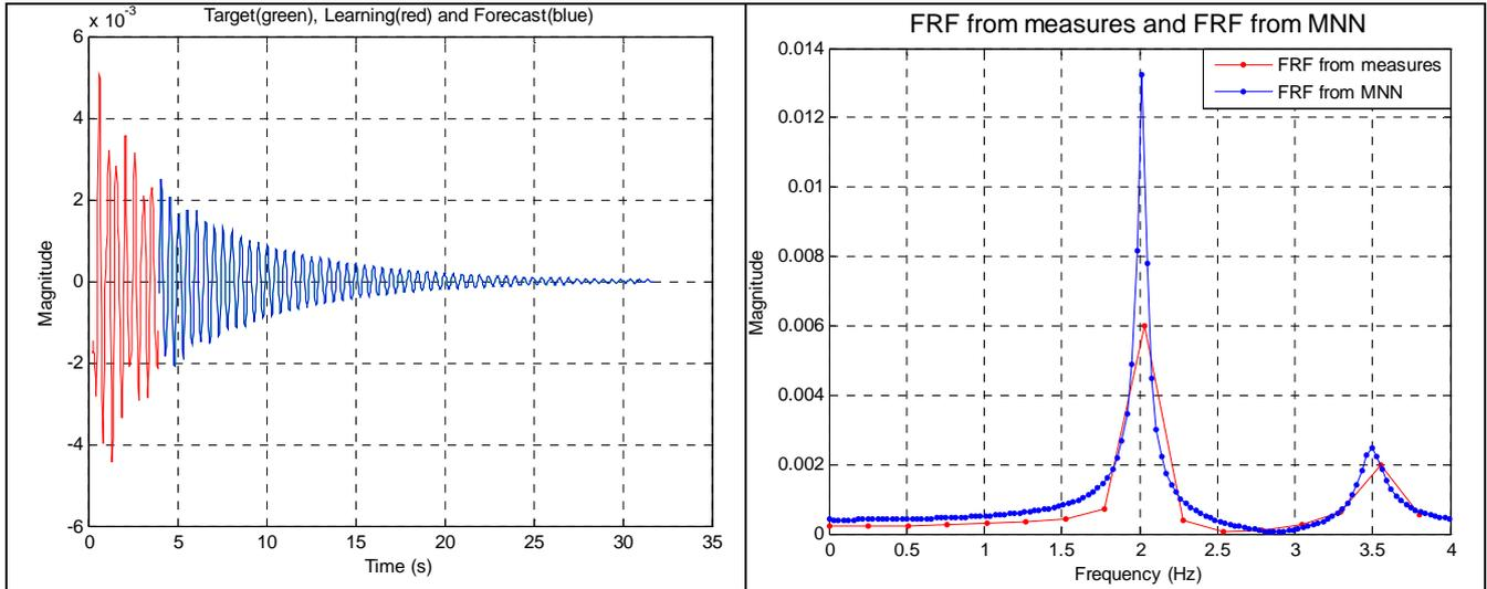
Figure 6- a) The signal that was improved via neural predictor; b) Comparison between both of the FRF.
