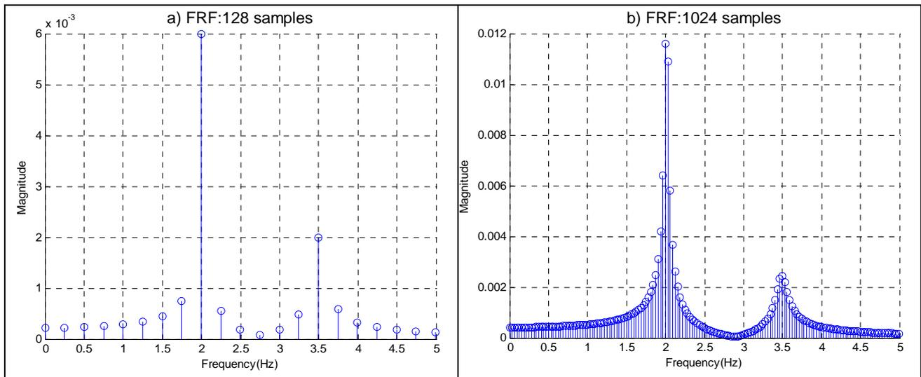
Figure 2. Discrete time FRF version: a) 128 samples; b) 1024 samples.
