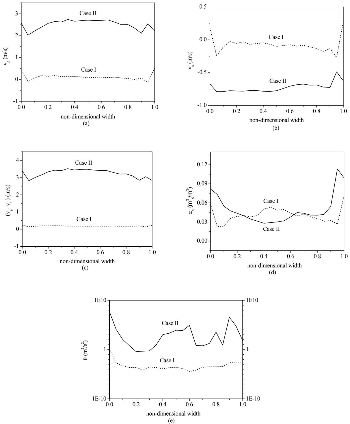
Figure 3. Time averaged profiles of gas axial velocity (a), solid axial velocity (b), slip velocity (c), solid volume fraction (d), and granular temperature (e) over the central line through a cross section of the domain at 4 cm above entrance.
