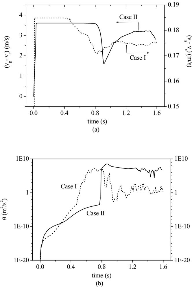
Figure 2. Transient behavior of parameters averaged over the whole domain, for cases I and II. (a) slip velocity; (b) granular temperature.
