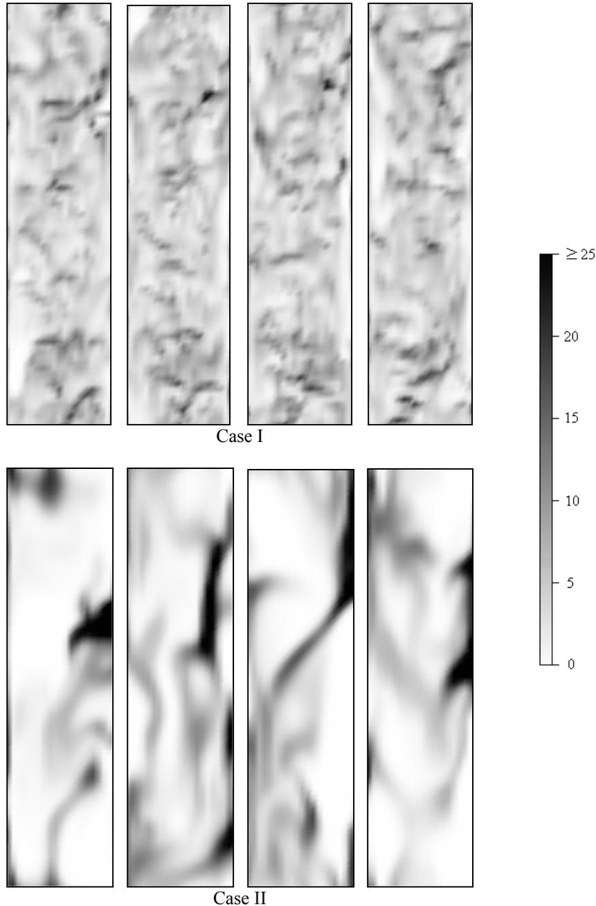
Figure 1. Grayscale plots of solid volume fraction in an axial section of the domain, for cases I and II (real scales).
