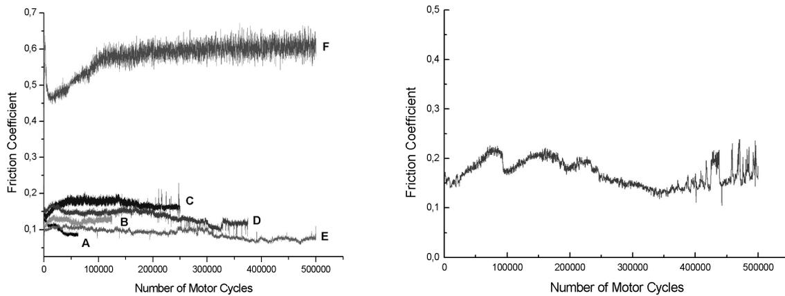
Figure 5. (a) Friction curve for some number of cycles. Curve from A to E – coated, curve F – uncoated. (b) Friction curve of 1 million cycles test, showing formation and consumption of transferred films.
