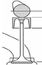
Figure 1. Tribosystem composed by cam of the command axle in contact with the valve lifter.
