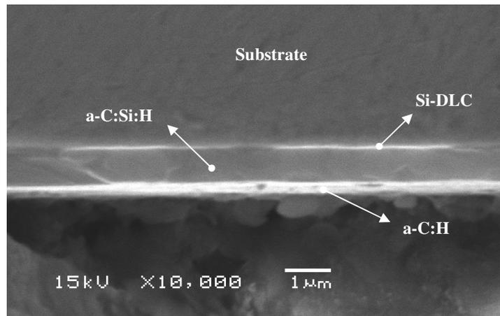
Figure 3. Scanning Electron Microscopy of the multilayer film.
