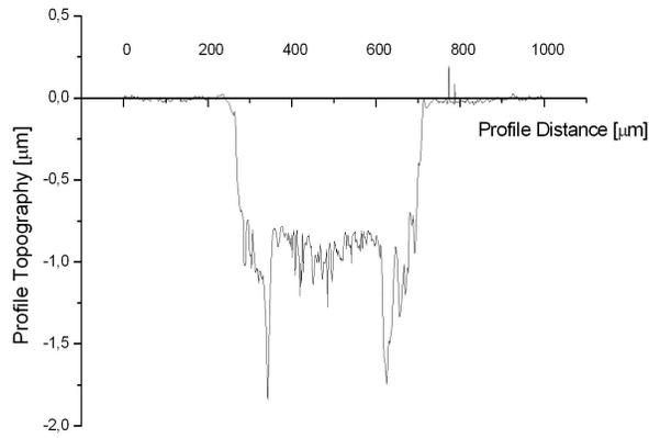
Figure 6. Perfilometry of groove formed while tribological test. 875000 cycles, Load = 10N, Hertzian contact = 1,42 GPa, V=5cm/s.
