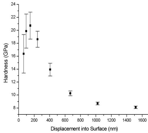
Figure 2. Dependence of film hardness value with depth from the surface
