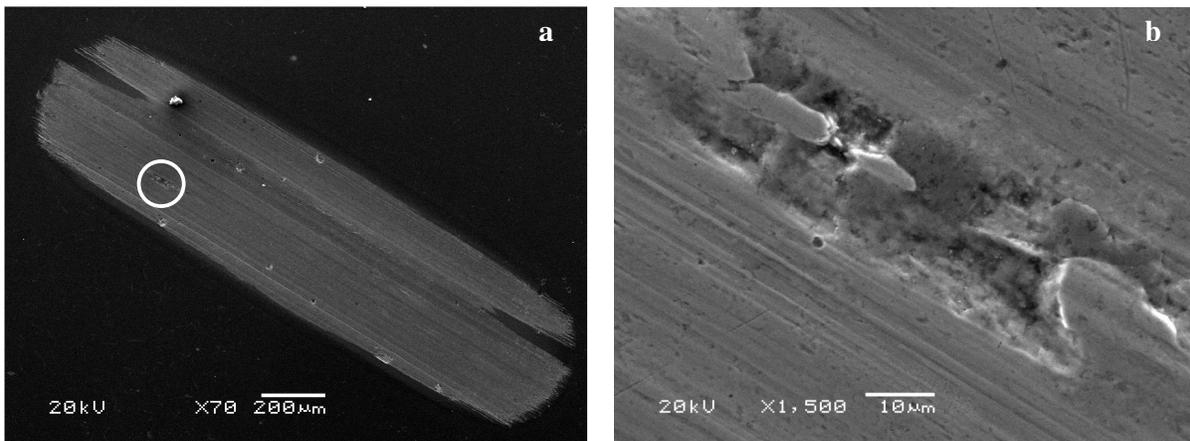
Figure 7. (a) Aspect of groove formed during the tribological test, (b) Detail of wear, suggesting film transference.
