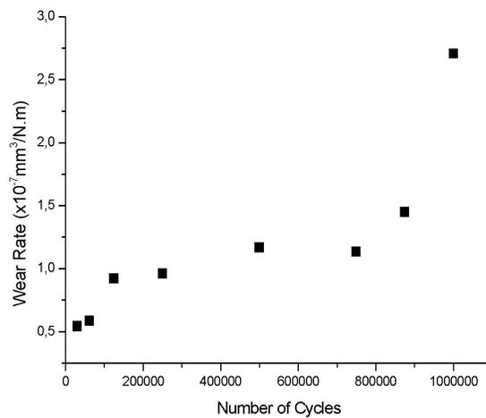
Figure 8. Wear curve for DLC + Si film
