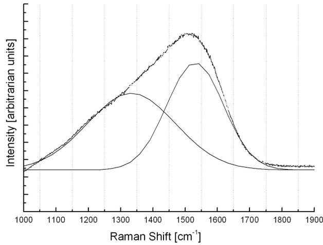
Figure 4. MW Raman spectroscopy for multilayer Si and DLC film
