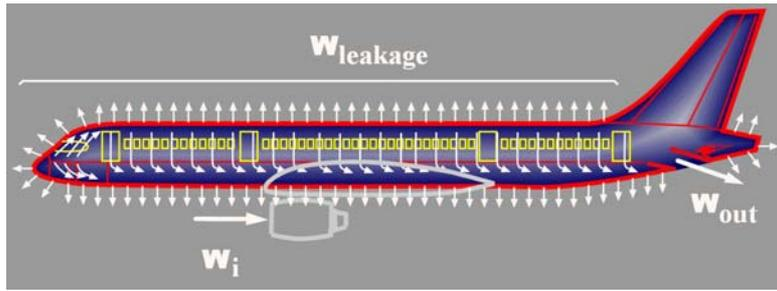
Figure 1 Schematic representation of the cabin mass balance parcels.
