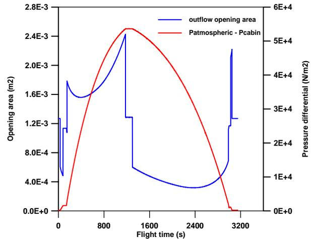
Figure 5 – Outflow valve opening area and pressure differential between atmospheric/cabin pressure.
