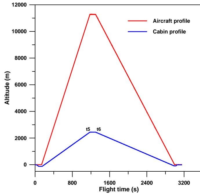
Figure 2 – Aircraft and cabin altitude profiles.
