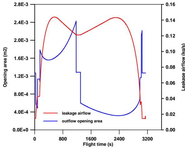
Figure 4 – Outflow valve opening area and cabin leakage airflow.
