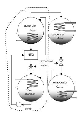
Figure 4 – Absorption cooling (AC) scheme.
