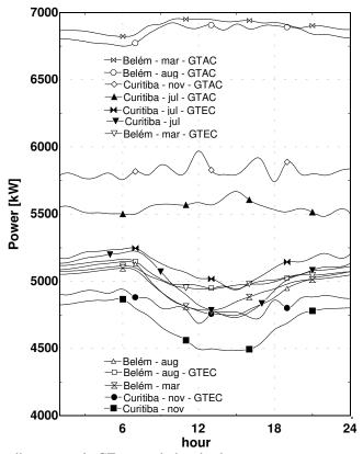
Figure 9 – Influence of the cooling-system in GT power during the day.
