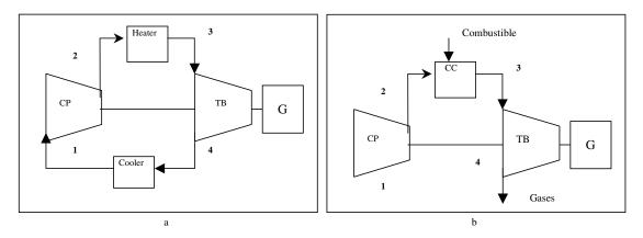
Figure 1 - a) Basic scheme of Brayton cycle. b) Basic scheme of gas turbine
