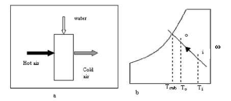
Figure 3 - a) Evaporative Cooling (EC) scheme. b) Evaporative cooling diagram of psychometric chart.
