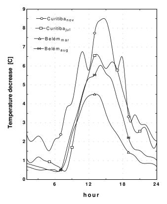
Figure 10 - Temperature decrease using EC in Belém and Curitiba.
