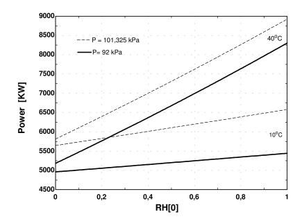
Figure 11 – Influence of the pressure, temperature and relative humidity in GTAC power.
