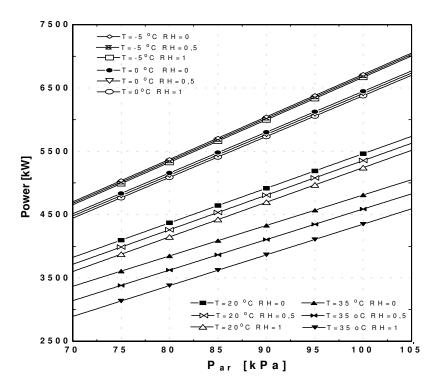
Figure 7 – Influence of inlet air pressure, temperature and relative humidity in the GT power.
