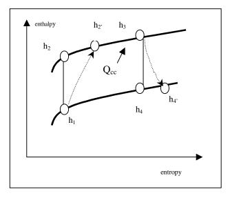
Figure 2 – Mollier diagram for air
