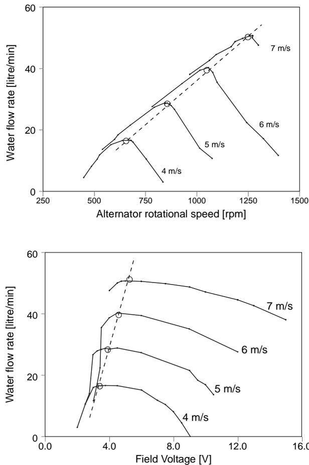
Figure. 3.- Water flow rate versus alternator speed and versus field voltage. The flow rate peaks have a linear variation with both variables.
