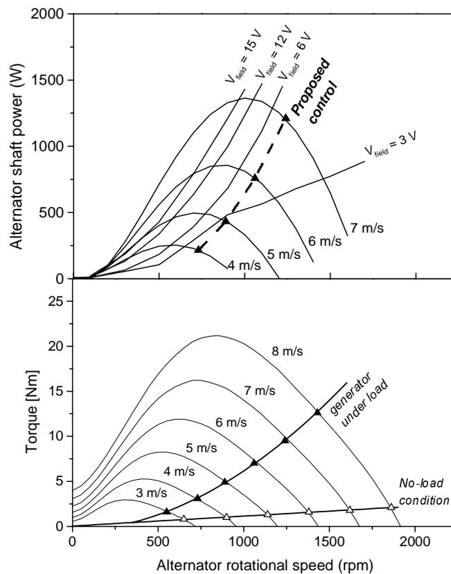
Figure 4 - Top: Mechanical power required to drive the alternator for different field voltages and power generated by the wind turbine at different wind speeds, vs. alternator rotational speed. Dashed line shows the power required with the proposed control. Bottom: Steady-state working points of the alternator in the presence of different wind speeds. Filled symbols: alternator feeding the pump; Empty symbols: alternator under no load condition.
