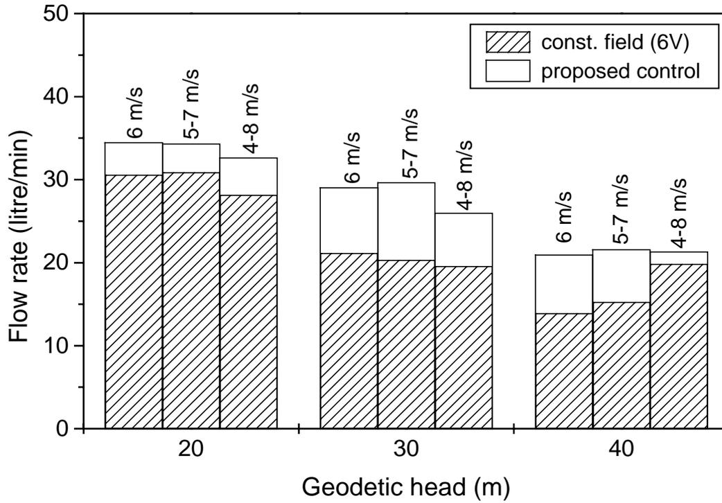
Figure 6 - Average water flow rate under the variable wind condition of Fig 5, obtained with constant field voltage (slashed bars) and with the proposed field voltage controller (white bars) for different geodetic heads.
