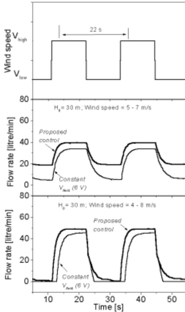
Figure 5- Top: Simulated wind condition. The wind speed varies between the values  $V_{high}$  and  $V_{low}$  with period = 22 s and duty cycle 50%.
