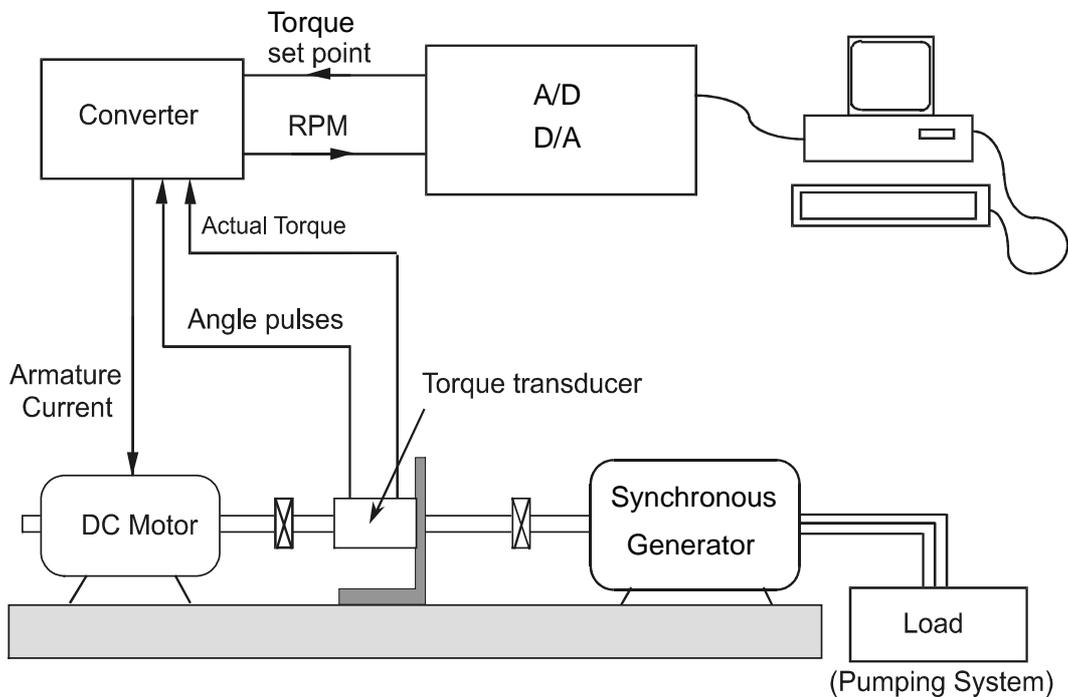
Figure 1. - Schematic diagram of the test-rig for components of a WECS
