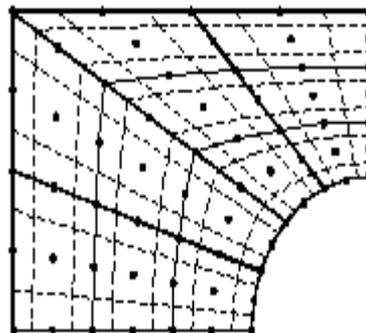
Figure 1 - Meshes of finite elements and control volumes
