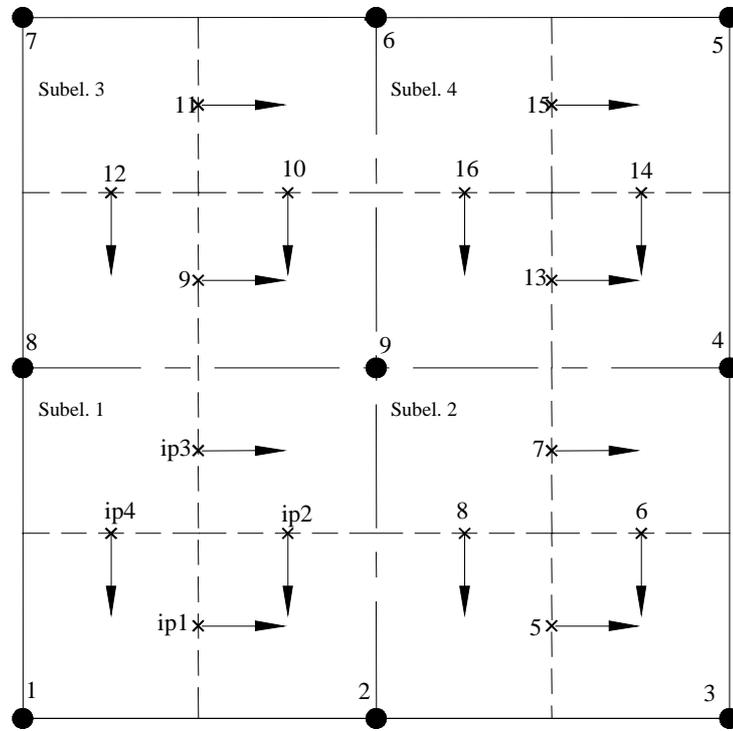
Figure 3 - Element for implementation of upwind
