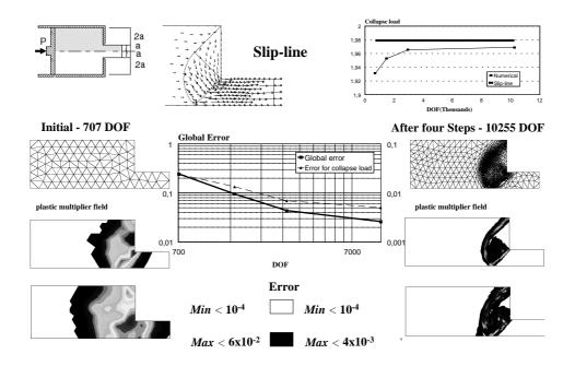
Figure 2: Frictionless extrusion through a square die.
