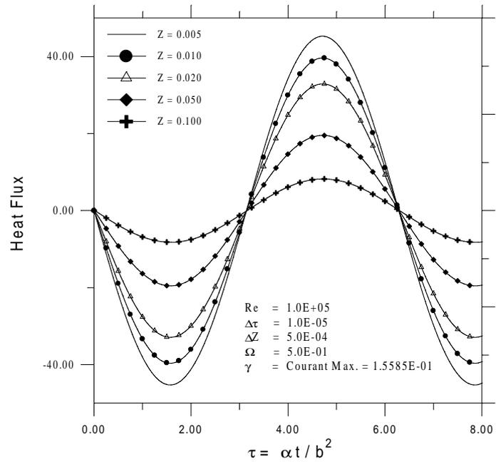
Figure 4b – Variation of the wall heat flux as a function of time for  $\Omega = 1.0$ .
