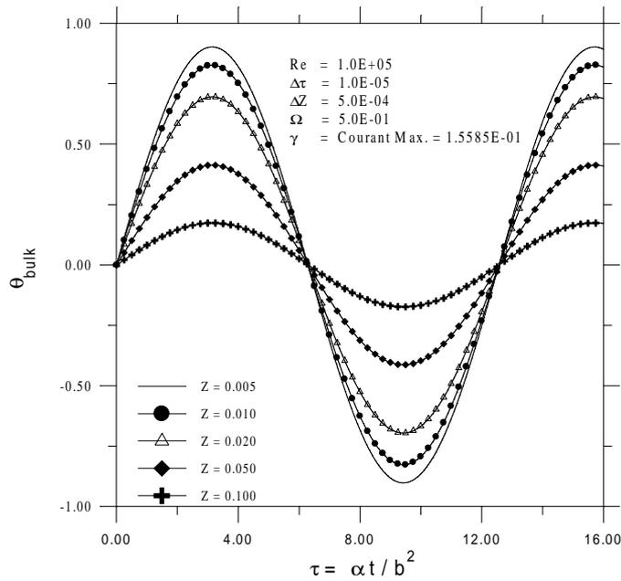
Figure 3a – Variation of the dimensionless bulk temperature as a function of time for  $\Omega = 0.5$ .
