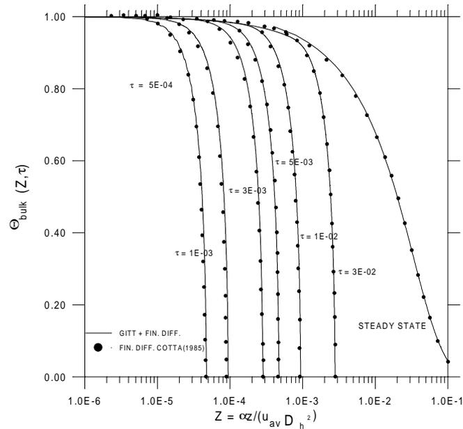
Figure 1 – Bulk temperature distribution in laminar flow for a step change in inlet temperature. Comparison with purely numerical solution in Cotta et al. (1986).
