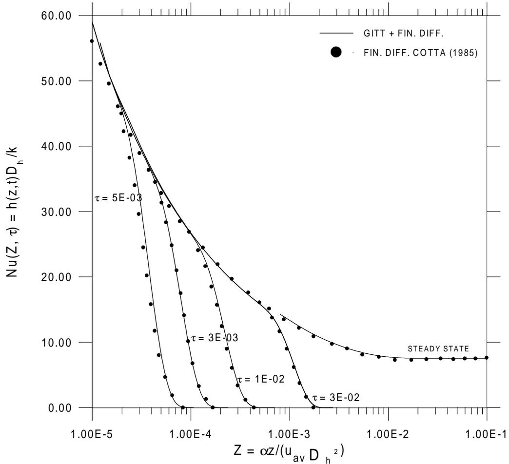
Figure 2 – Nusselt number distribution in laminar flow for a step change in inlet temperature. Comparison with purely numerical solution in Cotta et al. (1986).
