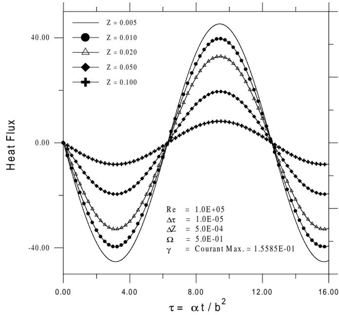
Figure 4a – Variation of the wall heat flux as a function of time for  $\Omega = 0.5$ .
