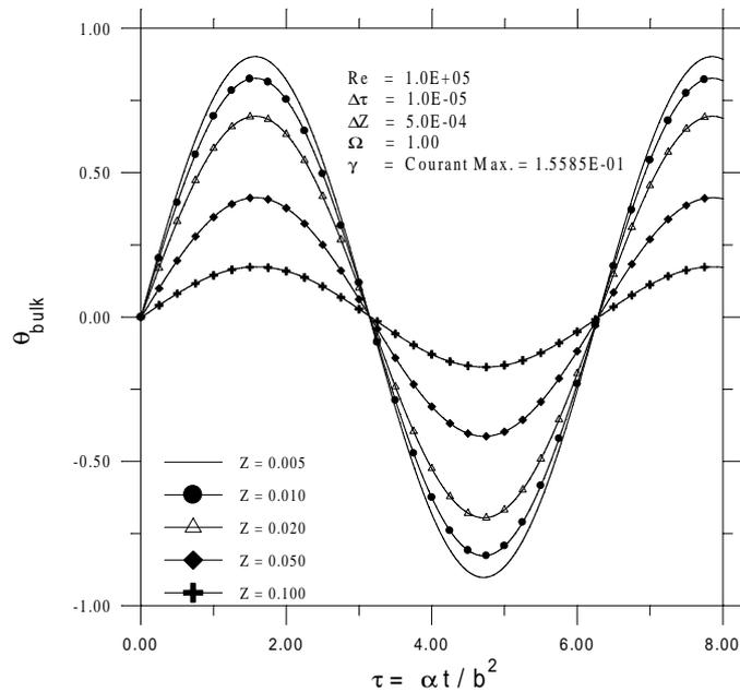
Figure 3b – Variation of the dimensionless bulk temperature as a function of time for  $\Omega = 1.0$
