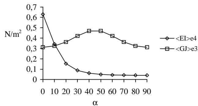
Figure 4 - Evolution of  $\langle EI \rangle$  and  $\langle GJ \rangle$  as function of the winding angle  $\alpha$  – kevlar/epoxy
