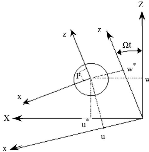
Figure 2 – The reference coordinate system of the shaft
