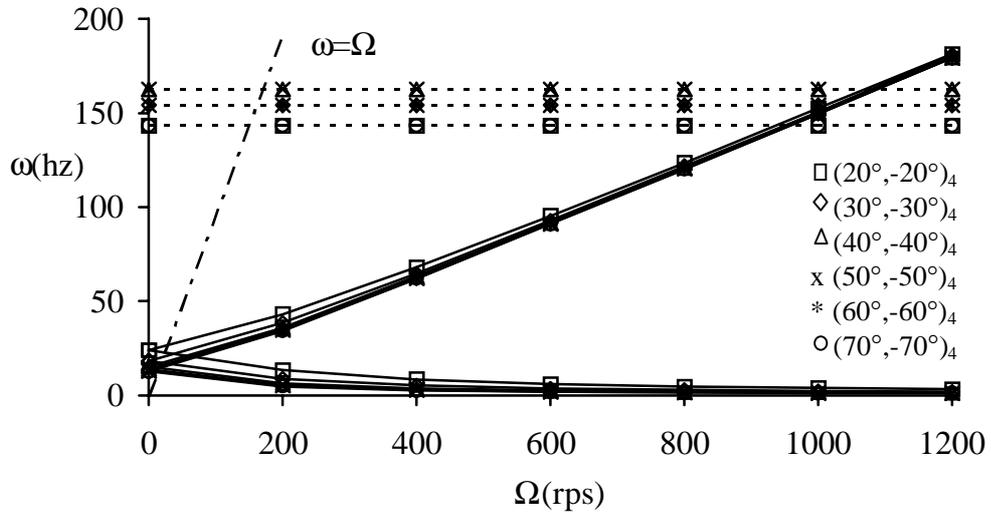
Figure 6 – Campbell Diagram - kevlar/epoxy winding shaft
