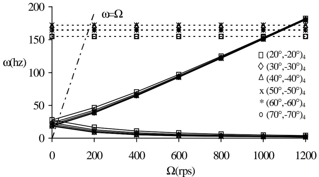
Figure 7 – Campbell Diagram - glass/epoxy winding shaft
