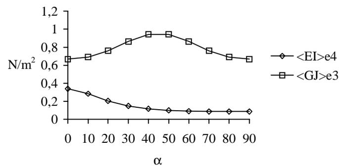
Figure 5 - Evolution of  $\langle EI \rangle$  and  $\langle GJ \rangle$  as function of the winding angle  $\alpha$  – glass/epoxy
