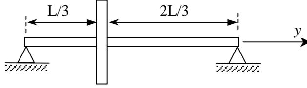
Figure. 3 – Rotor simple-supported on the ends
