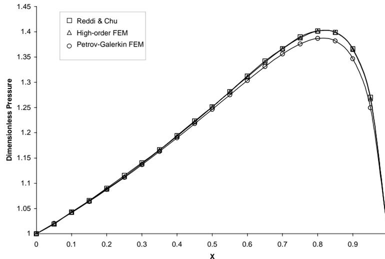
Figure 2 – Comparative results for dimensionless pressure on a plane slider bearing.
