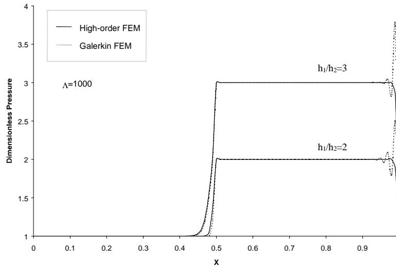
Figure 6 – Numerical oscillations at the trailing edge of Rayleigh step bearings ( $L_1/L_2=1$ ).
