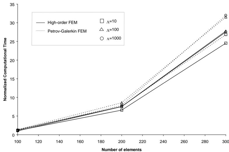
Figure 5 – Comparative computational efficiency for a Rayleigh step bearing ( $h_1/h_2=2$ ,  $L_1/L_2=1$ ).
