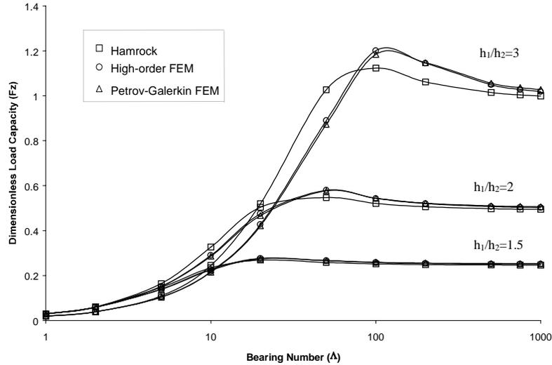
Figure 3 – Dimensionless bearing load capacity for Rayleigh step bearings ( $L_1/L_2=1$ ).
