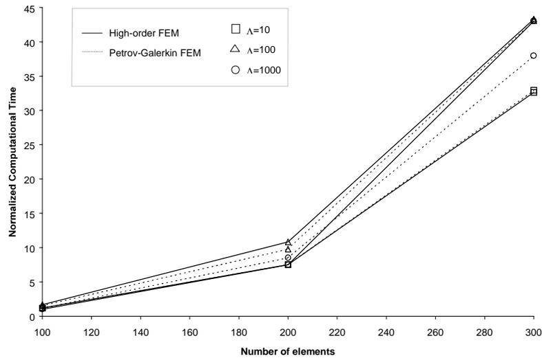
Figure 4 – Efficiency of the FEM procedures for a plane slider bearing ( $h_1/h_2=3$ ).
