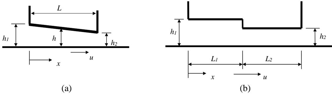
Figure 1 – Schematic views of a plane slider bearing (a) and a Rayleigh step bearing (b).
