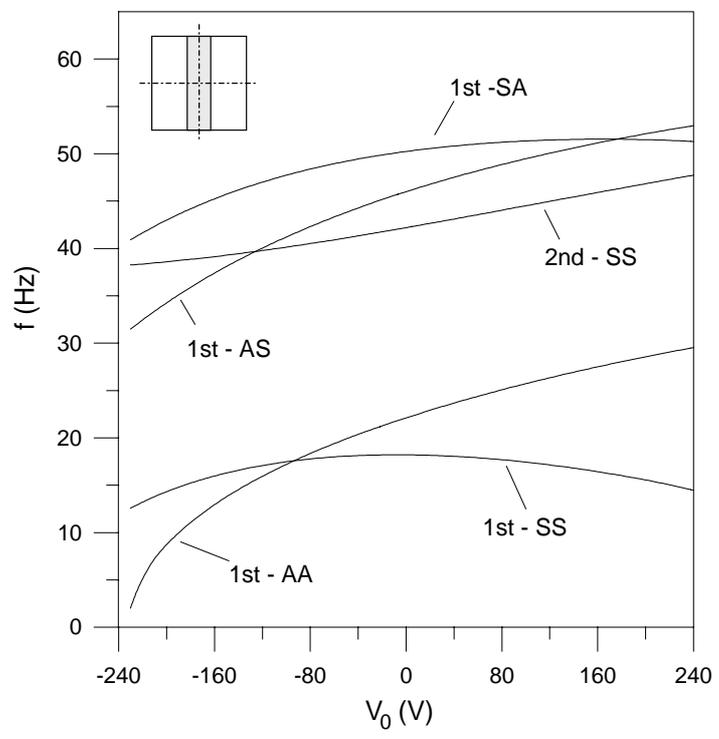
Figure 3 - Natural frequency as a function of voltage for actuators at the center
