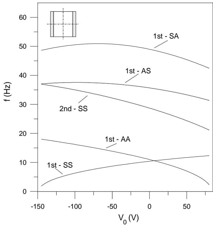
Figure 2 - Natural frequency as a function of voltage for longitudinal actuators at the edges
