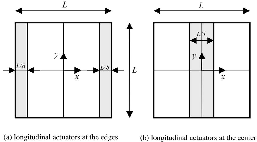
Figure 1 - Piezoelectric actuator configurations
