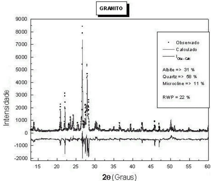
Figure 1- Diffractogram of “Asa Branca” Granite
