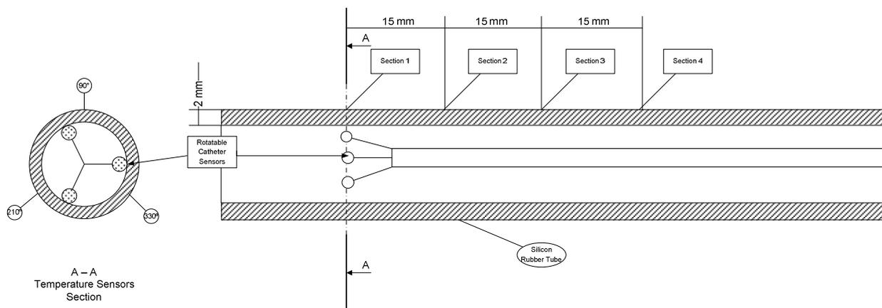
Figure 1. Experimental setup showing the vessel model, temperature sensors positions at the outer wall and the temperature sensing catheter.
