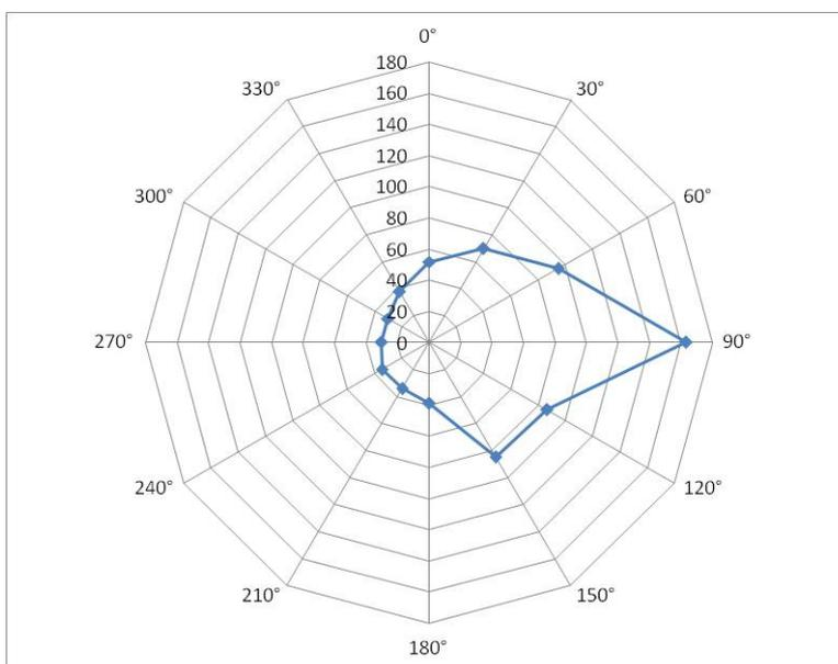
Figure 3. Maximum temperatures (radial coordinate in °C) measured at the inner wall of the vessel as a function of the angular orientation (angular coordinates). 90° corresponds to the upper part of the vessel.
