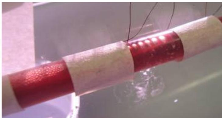
Figure 2. Small bubbles formation at the tip of the laser fiber (left side) and downstream agglomeration into larger bubbles (right side).
