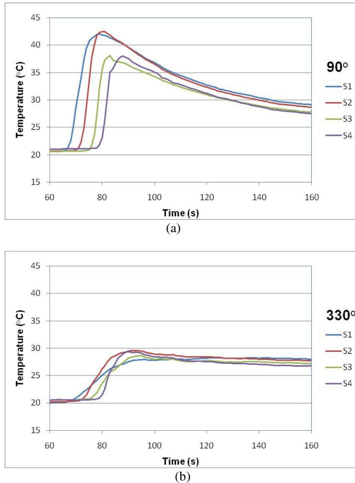
Figure 4. Outer wall temperature histories for 90° and 330° angular orientations for the four measurement sections (S1 to S4).
