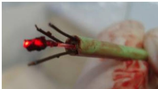
Figure 5. Presence of blood clots at the fiber tip after a typical test.
