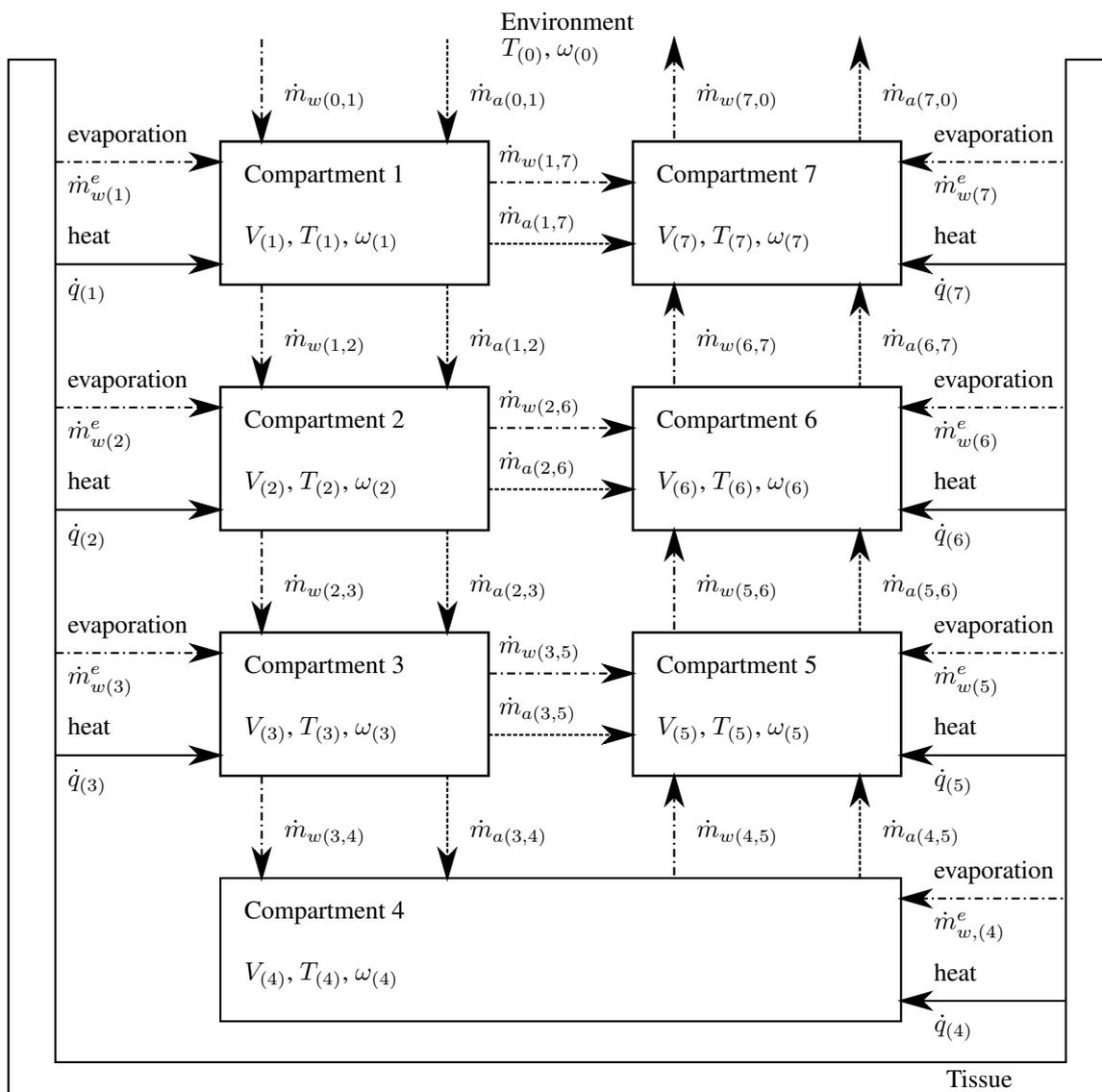
Figure 1. Compartment model description. The arrows represent the heat from the tissues to the compartment (solid line), the dry air flow between compartments (dashed line), and the water vapor flow between compartments and from the evaporation (dash-dot line).
