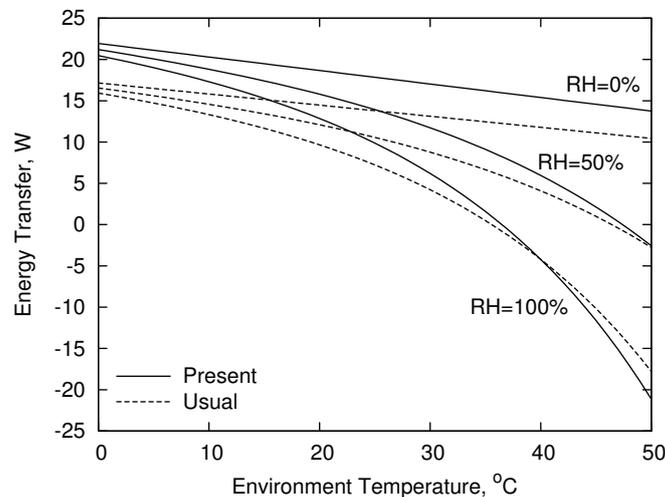
Figure 2. Comparison of energy transfer through the respiratory tract obtained by the present model and the usual methodology proposed by Fanger (1970), for relative humidity equal to 0%, 50% and 100%. The tissue temperature was set to 37 °C and the pulmonary ventilation to 8 L/min.
