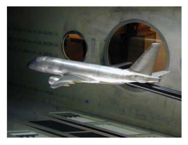
Figure 10. Transonic pressurized tunnel test - EMBRAER 170 at DNW/HST.
