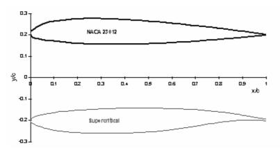
Figure 20. Typical geometry - Conventional and supercritical airfoils.
