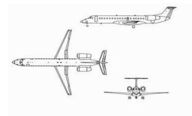
Figure 21. ERJ145 - Rear fuselage mounted engines configuration.
