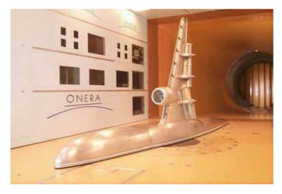
Figure 8. Subsonic pressurized tunnel test - EMBRAER 170 half model at ONERA F1.
