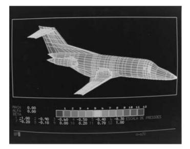
Figure 2. Early 3D panel method pressure distribution results (CBA123 model).
