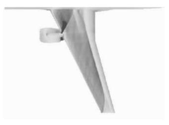
Figure 5a. CFD pressure distribution results for wing-pylon-nacelle configuration (EMBRAER 170) Initial configuration with wing upper surface shock caused by pylon-wing interference.
