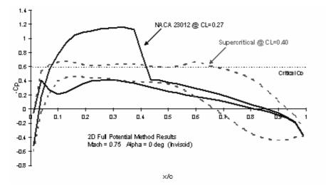
Figure 19. Typical pressure distributions - Conventional and supercritical airfoils.
