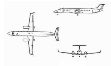
Figure 17. ERJ145 - Over wing mounted engines configuration.
