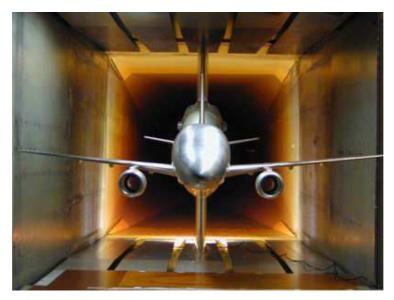
Figure 11. Transonic pressurized tunnel test - EMBRAER 170 at DNW/HST - Front View.
