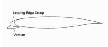
Figure 22. ERJ145 leading edge droop and vortilons.
