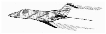
Figure 1. Early 3D panel method mesh (CBA123 model).
