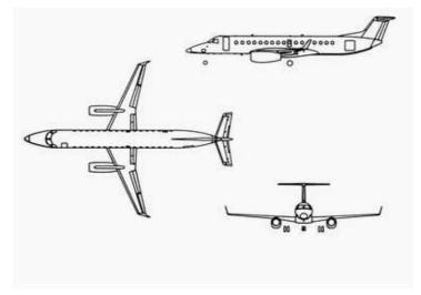
Figure 18. ERJ145 - Under wing mounted engines configuration.
