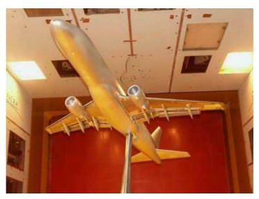
Figure 9. Subsonic pressurized tunnel test - EMBRAER 170 full model at ONERA F1.
