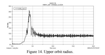
Figures 13(a) and 14 are two ways to show the behavior of the upper orbit. Figure 13(b) shows the behavior of the lower orbit. During the transient the radius of the orbit is bigger than during the steady state. With these data we can check if the tub will hit the cabinet and have an idea of the vibration level during the steady state.
