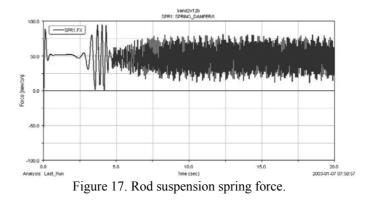
The force in the rod suspension spring during the steady state is very useful to predict the vibration transmitted to the cabinet. As bigger the amplitude force as bigger will be the cabinet vibration.
