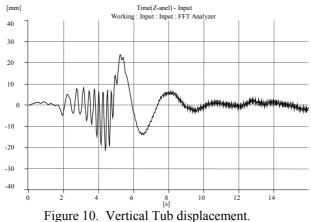
Figure 10 shows the vertical displacement of the tub in the point 3. This kind of result is useful to check hitting of the tub with the top of the machine or components assembled on the top.
