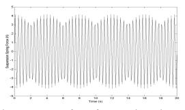
Figure 5. Response force of a suspension spring.
