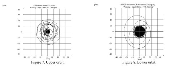
Figure 7 shows the behavior of the upper orbit. Figure 8 shows the behavior of the lower orbit. During the transient the radius of the orbit is bigger than during the steady state. With these data we can check if the tub will hit the cabinet and have an idea of the vibration level during the steady state.
