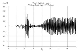
Figure 11. Vibration of the lateral panel of the cabinet (point 4).
