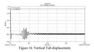
Figure 16 shows the vertical displacement of the tub. This kind of result is useful to check hitting of the tub with the top or components assembled on the top.
