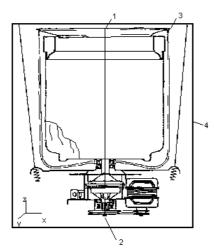
Figure 6. Points in the washing machine to get information
