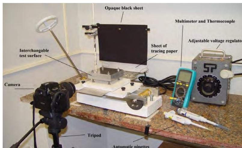
Figure 2. Experimental bench developed to measure contact angle of droplets onto different surfaces and instruments used to acquire the data.
