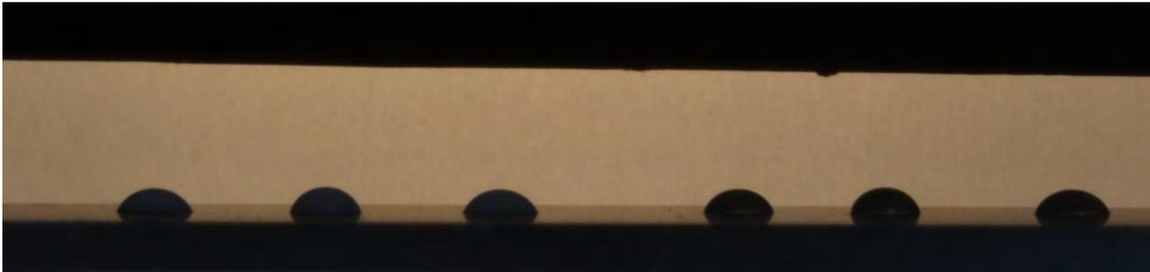
Figure 3: Six droplets of nanofluid over the test surface. Picture taken using the experimental bench developed in the present study.
