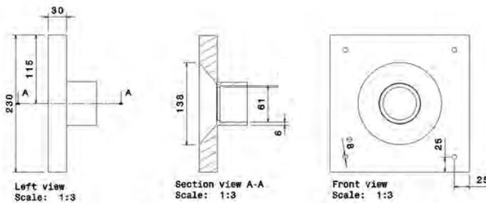
Figure 4(a). Acoustic box cover dimensions in mm.
