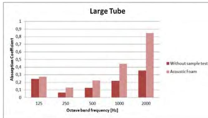
Figure 12. Absorption coefficient estimated with the large tube.
