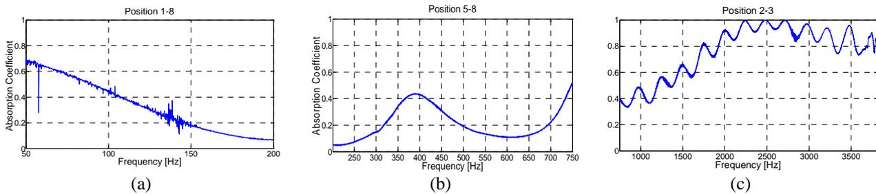
Figure 11. Absorption coefficients curves estimated for the egg crate pattern acoustic foam using the large-duct.
