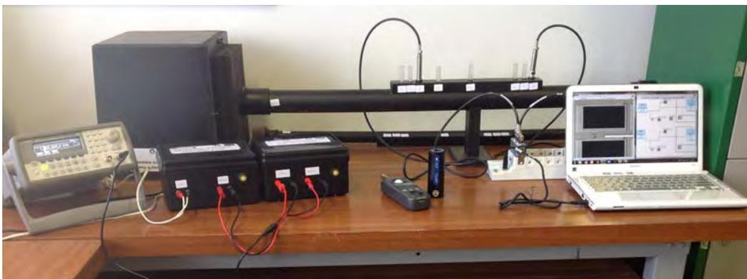
Figure 8. Acoustic impedance tube measurement setup: Two microphones technique.
