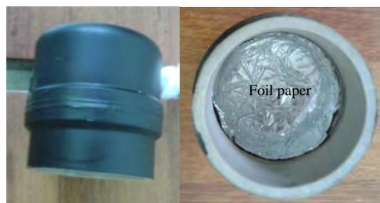
Figure 5(b). Sample holder (side view) and foil paper coating.
