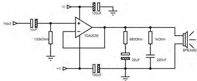
Figure 6. Power amplifier circuit.
