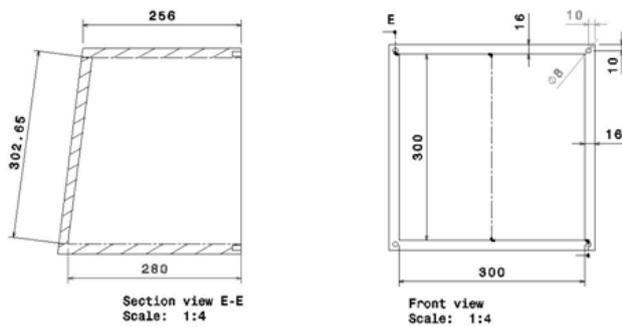
Figure 3(a). Acoustic box dimensions in mm.
