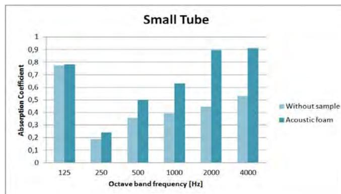
Figure 13. Absorption coefficient estimated with the small tube.
