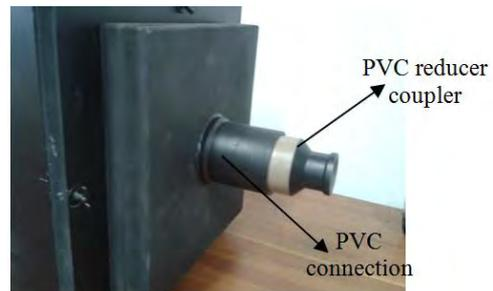
Figure 4(b). Detail of PVC reducer coupler.
