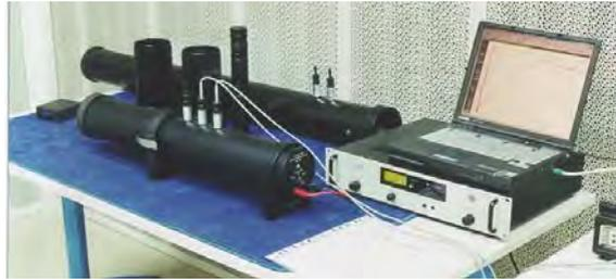
Figure 9. Commercial acoustic impedance tube measurement setup (Source: Bruel & Kjaer).
