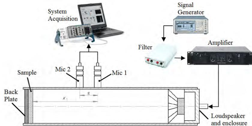
Figure 1. Impedance tube setup.
