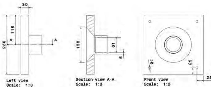
Figure 4(a). Acoustic box cover dimensions in mm.
