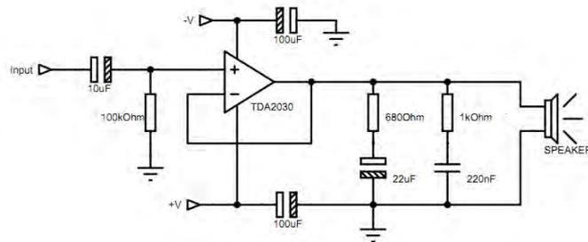
Figure 6. Power amplifier circuit.
