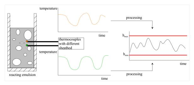
Figure 1. Strategy for monitoring of convection coefficient
