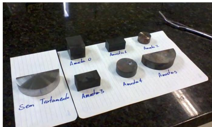
Figure 2. Samples used for heat treatment
