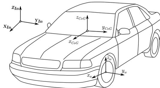
Figure 3. Reference Systems in Vehicle Dynamics.
