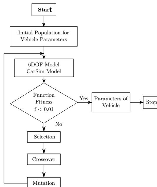
Figure 7. Flow chart for vehicle parameter estimation.
