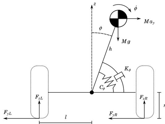
Figure 5. Vehicle Roll Model, suspension are modeled as a torsional spring and damper.
