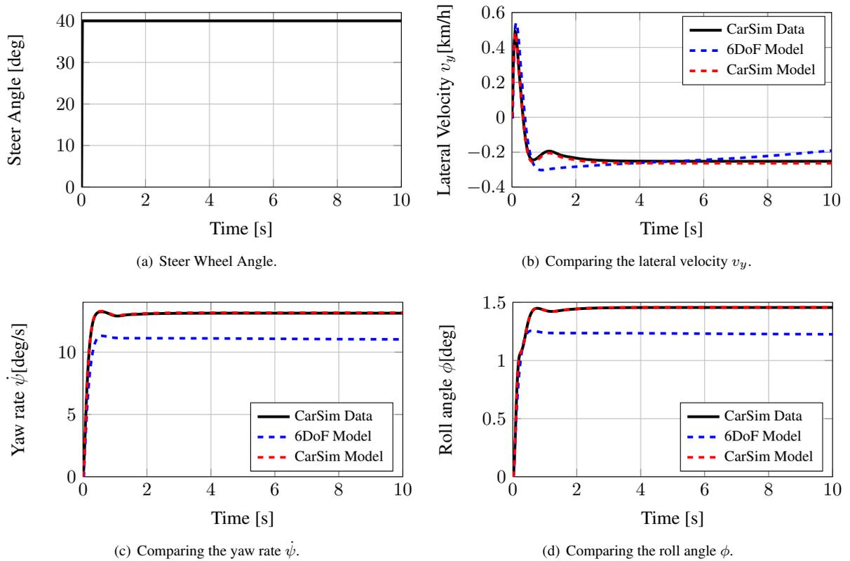
Figure 8. Comparing between real data, 6DOF estimation and CarSim model estimation for step steer.
