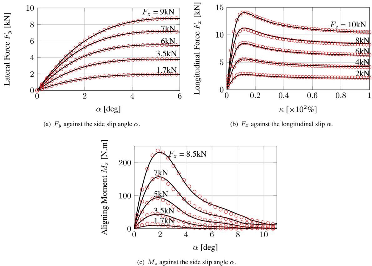
Figure 2. Real data CarSim (solid lines) versus optimized Magic Formula (red circles).
