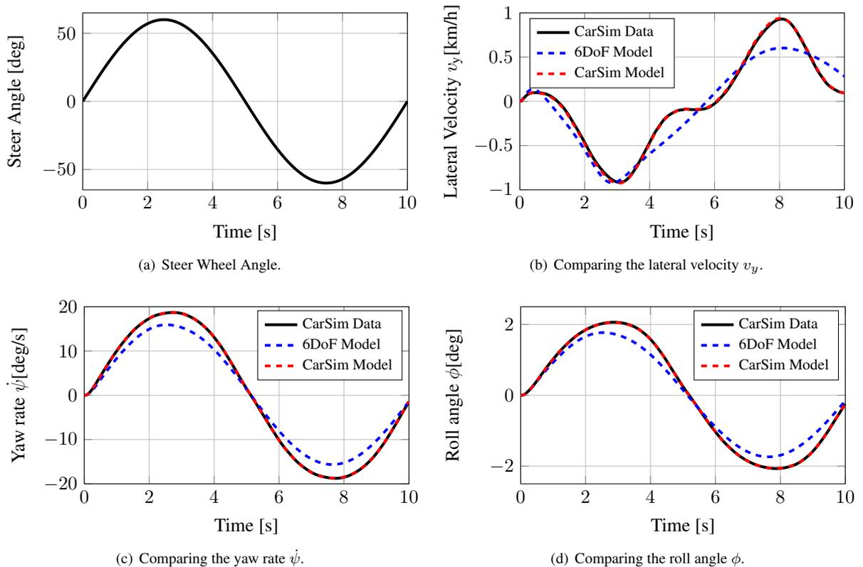
Figure 9. Comparing between real data, 6DOF estimation and CarSim model estimation for sinusoidal steer.
