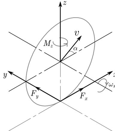
Figure 1. Diagram of a wheel showing its local axis, the forces acting at the contact point, the angular velocity  $\omega$  and the total velocity  $v$ .
