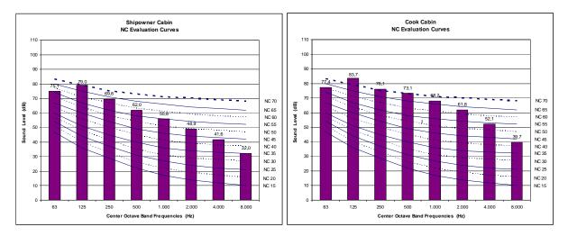
Figure 4. Octave band spectra of the sound level in the shipowner cabin and in the cook cabin, superposed to the NC curves from NBR 10152:1987.
