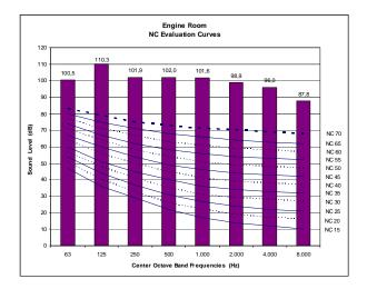
Figure 6. Octave band spectra of the sound level in the engine room superposed to the NC curves from NBR 10152:1987.
