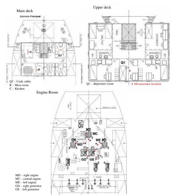
Figure 2. Measurement locations in the superstructure of the ship
