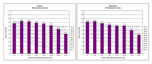
Figure 5. Octave band spectra of the sound level in the kitchen and in the mess room superposed to the NC curves from NBR 10152:1987.
