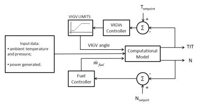
Figure 1. Block diagram of the implemented control system.
