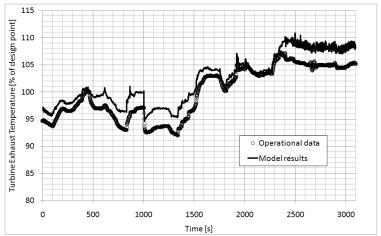
Figure 5. Comparison of turbine exhaust temperature transient simulated and engine data.
