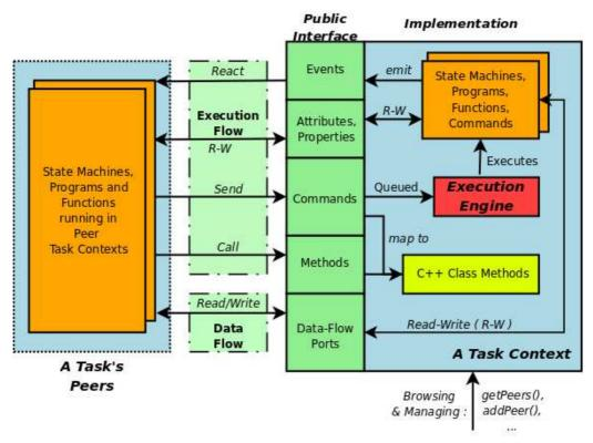
Figure 6. Interface of a component(Soetens, 2009).
