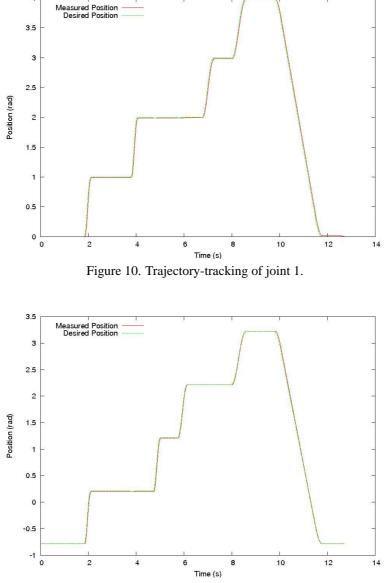
Figure 11. Trajectory-tracking of joint 2.
