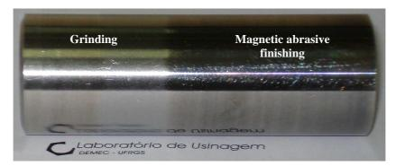
Figure 8. Surface quality obtained through grinding and magnetic abrasive finishing.
