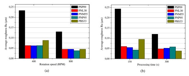
Figure 5. Variation of surface roughness for different oils as a function of: (a) rotation speed; and (b) processing time.
