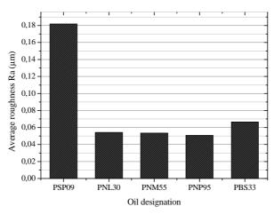
Figure 4. surface roughness Ra obtained with tested oils.
