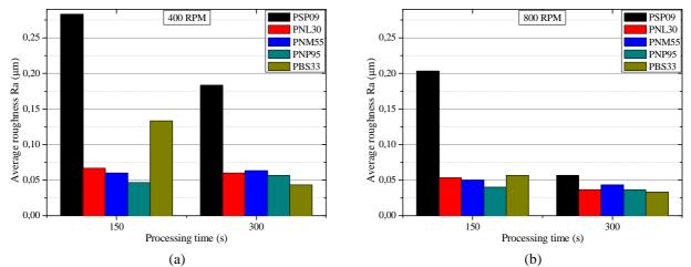
Figure 7. Average roughness obtained for magnetic abrasive powders containing different oils at (a) 400 RPM; and (b) 800 RPM.
