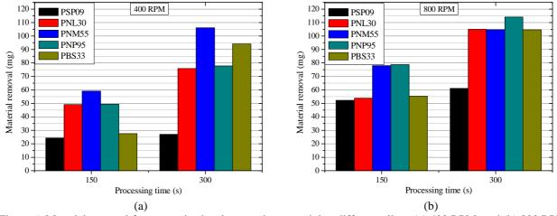
Figure 6. Material removal for magnetic abrasive powders containing different oils at (a) 400 RPM; and (b) 800 RPM.
