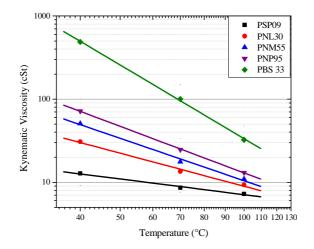
Figure 2. Viscosity as a temperature function for studied oils.
