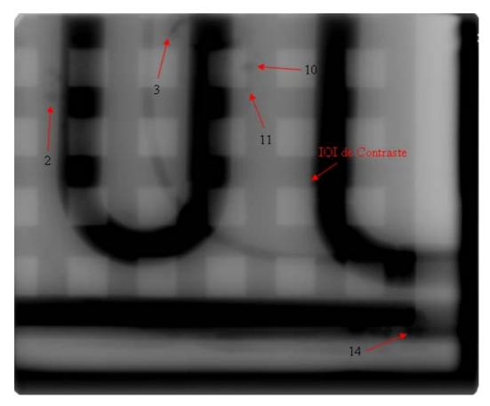
Figure 6. Image obtained with a class 2 film showing discontinuities in the areas of greater thickness.
