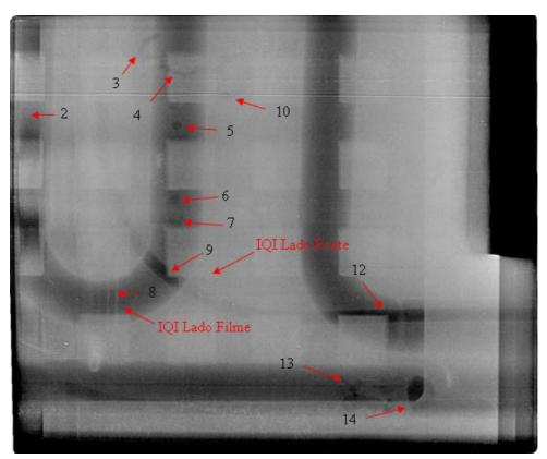
Figure 11. Industrial computed radiography using Cobalt-60.
