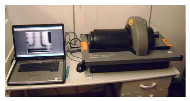
Figure 3. Industrial computed radiography equipment GE CR50P.
