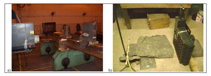
Figure 5. Experimental setup for radiographic testing - a) Linear Accelerator b) Cobalt-60.
