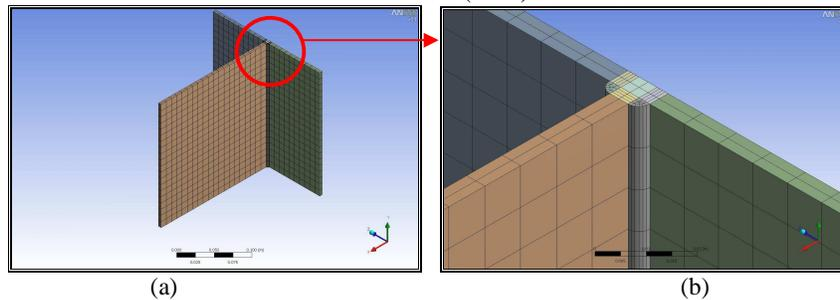
Figure 8. Coarse mesh: Solid 1 and 2 mesh (a) and detail of the weld zone (b).
