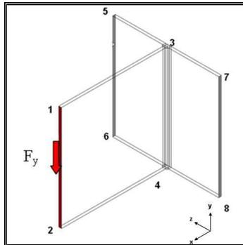
Figure 7. Loading and boundary conditions.
