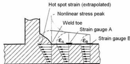
Figure 2. Measurement of the hot spot strain range using linear extrapolation method (Niemi, 1995).
