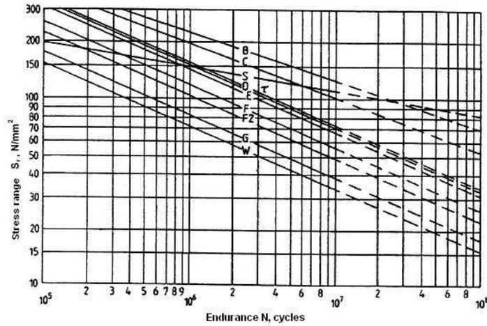
Figure 3. Fatigue life curve to each welded joint class (BS7608, 1993).
