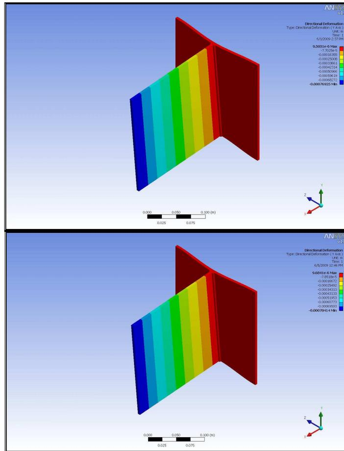
Figure 12. Displacement UY (m) Solid 1 (top) and Solid 2 (bottom).
