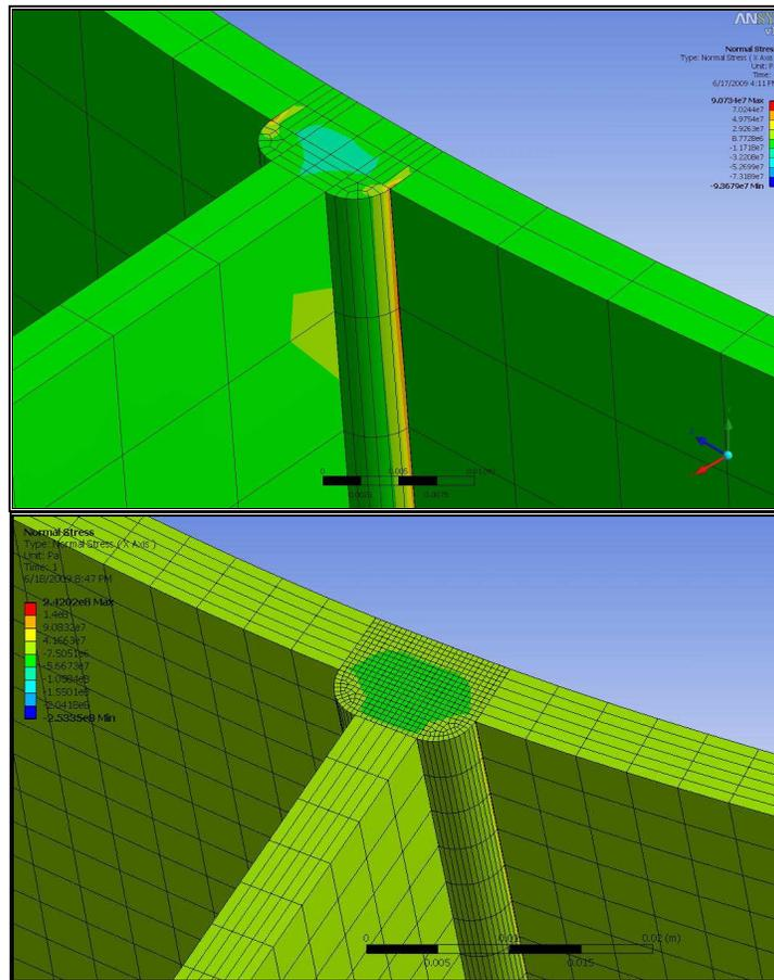
Figure 16. Solid 2 Normal Stress (Pa)  $\sigma_x$  (with frictional contact) – detail of welded location. Coarse mesh (top) and refined mesh (bottom).
