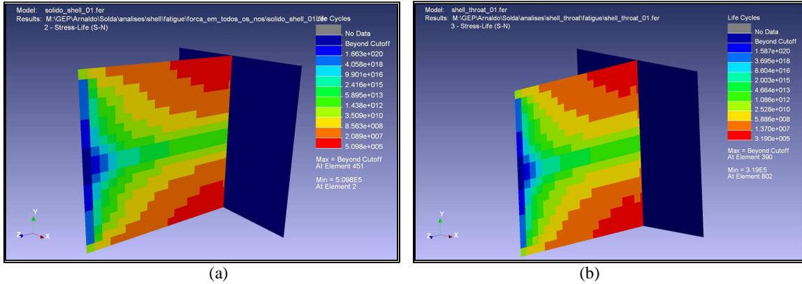
Figure 17. Fatigue Life (cycles) to Shell 1 – simply connected at the joint location – (a) and Shell 2 – double sided throat thickness – (b) (Alexandre et al, 2001).
