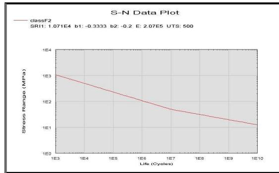
Figure 5. Stress-Life curve (logS x logN) to class F2.
