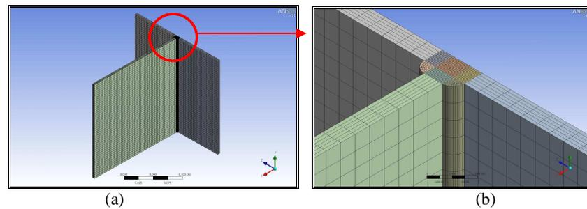
Figure 9. Refined mesh: Solid 1 and 2 mesh (a) and detail of the weld zone (b).
