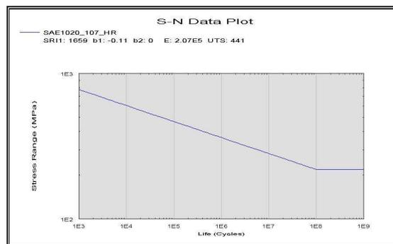
Figure 4. Stress-Life curve ( $\log S \times \log N$ ) to SAE1020.
