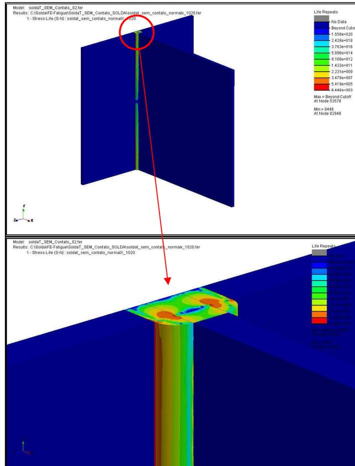
Figure 18. Fatigue Life (cycles) – Solid O1 (no contact) - refined mesh (top) and detail of weld location (bottom).
