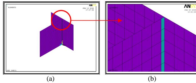
Figure 10. Shell 1 and 2 mesh (a) and detail of the throat thickness in the weld zone (b) (Alexandre et al, 2001).
