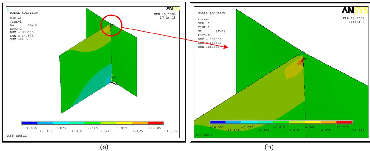
Figure 13. Normal Stress (MPa)  $\sigma_z$  to shell 1 model (a) and detail of weld location (b) (Alexandre et al, 2001).
