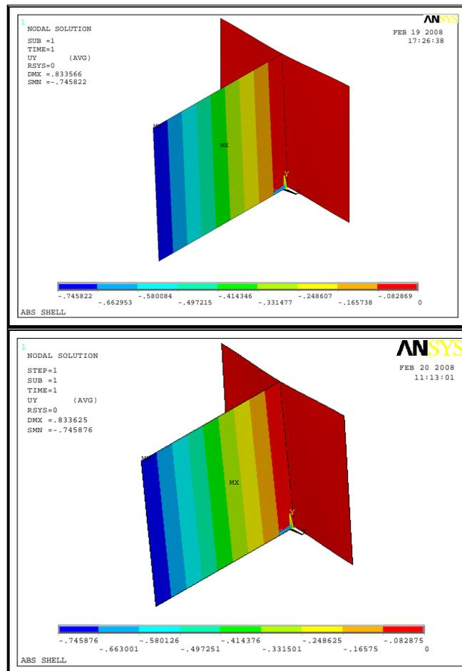
Figure 11. Displacement UY (mm) Shell 1 (top) and Shell 2 (bottom) (Alexandre et al, 2001).
