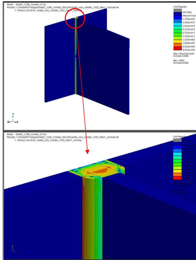
Figure 19. Fatigue Life (cycles) – Solid O2 (friction contact) - refined mesh (top) and detail of weld location (bottom).
