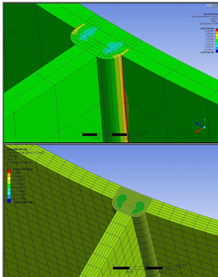
Figure 15. Solid 1 Normal Stress (Pa)  $\sigma_x$  (without contact) – detail of welded location. Coarse mesh (top) and refined mesh (bottom).
