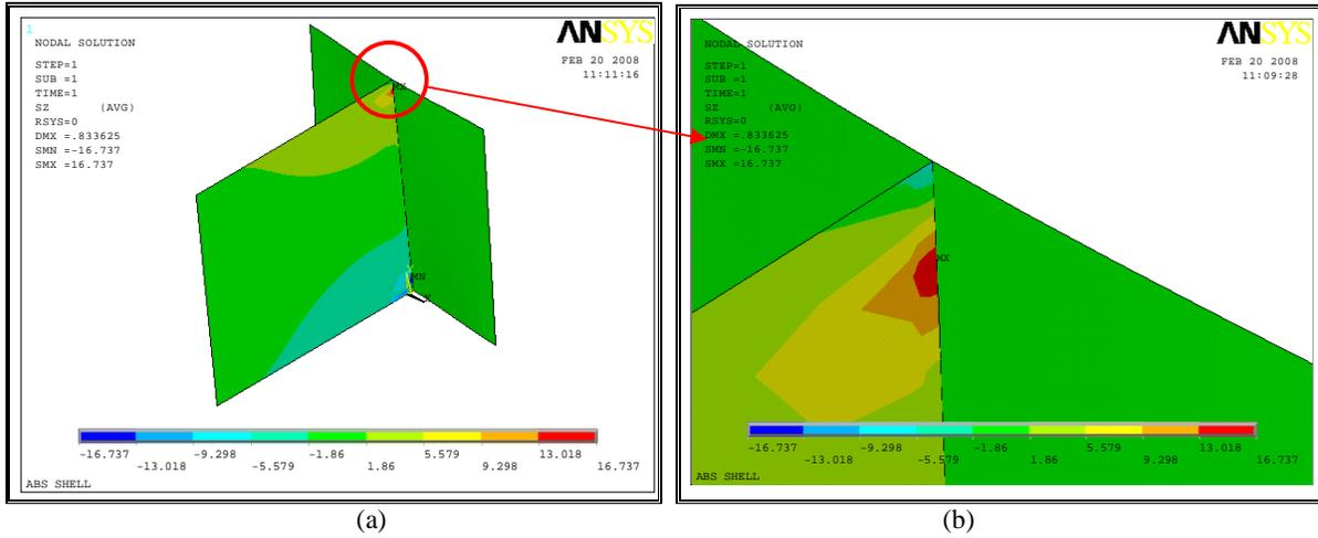
Figure 14. Normal Stress (MPa)  $\sigma_z$  to shell 2 model (a) and detail of weld location (b) (Alexandre et al, 2001).
