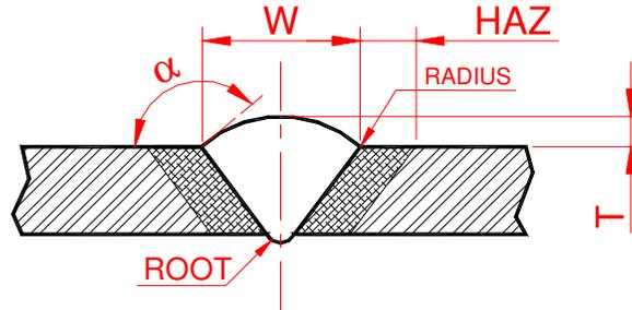
Figure 5: Principal geometric factors from weld profile.
