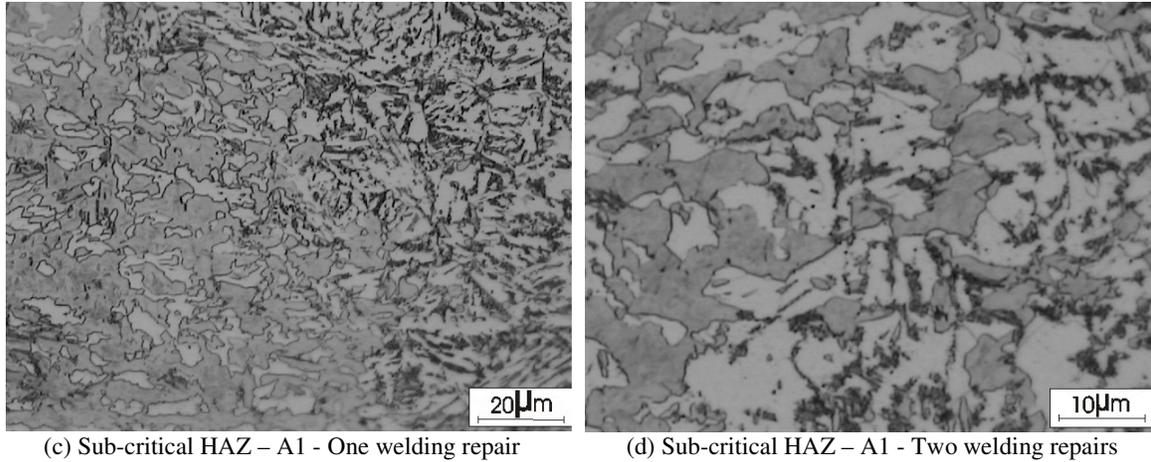
Figure 6: Base-material and base-material/HAZ transition microstructures. Nital 2%.
