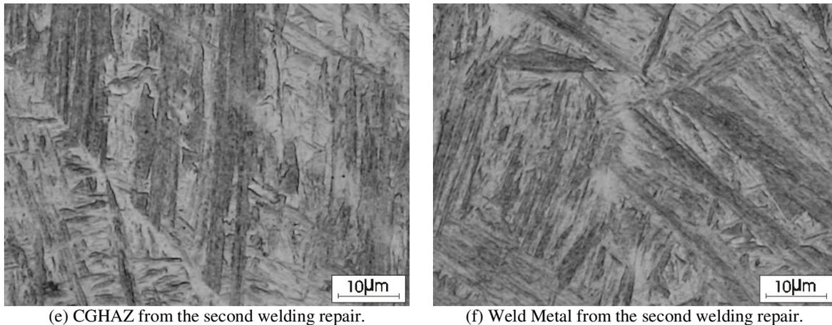
Figure 7: Microscopic analysis from the welding regions. Nital 2%.
