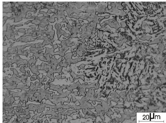
(b) Sub-critical HAZ – A1 – Original weld.
