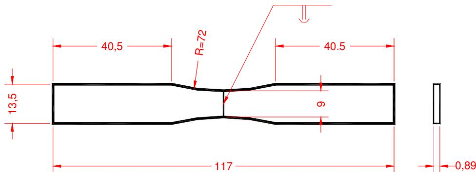
Figure 3: Axial fatigue specimen [mm].
