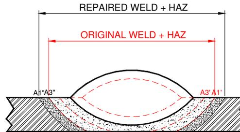
Figure 2: Repair welding process by overlapping the previous weld metal.
