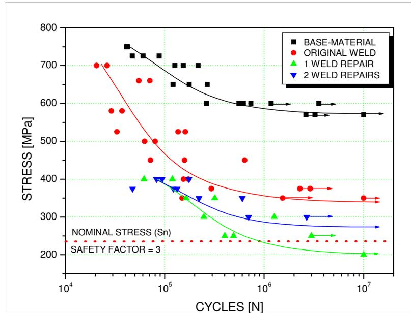
Figure 4: SN axial fatigue curves from base-material and welded specimens subjected to one and two welding repairs.
