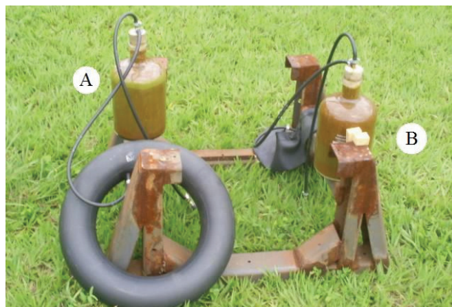
Figure 3. Biodigester and gasometer after seven days of biodigestion.
