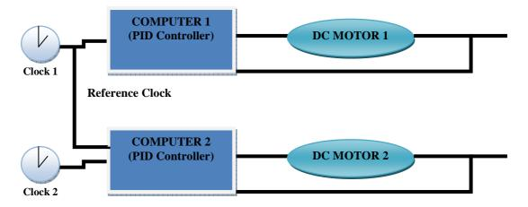
Figure 1. Parallel Control System.
