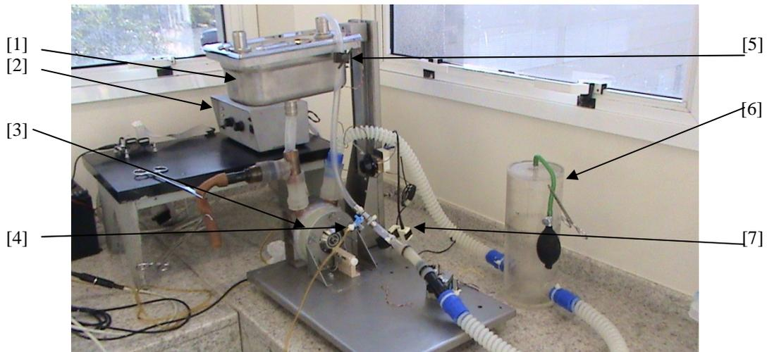
Figure 2. Assembled system: [1] Reservoir; [2] Electronic controller; [3] BLDC Pump; [4] Pressure Probe; [5] Tourniquet; [6] Compliance chamber; [7] Flow Probe.
